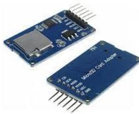
**Gambar 2.7 SD card adapter module**
