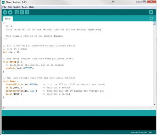
The image shows a screenshot of the Arduino IDE interface. The window title is "Blink | Arduino 1.0.5". The menu bar includes "File", "Edit", "Sketch", "Tools", and "Help". Below the menu bar is a toolbar with icons for file operations and execution. The main text area contains the following code:
