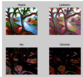
Gambar 1.4. Komponen Luminance, Hue, Saturation
