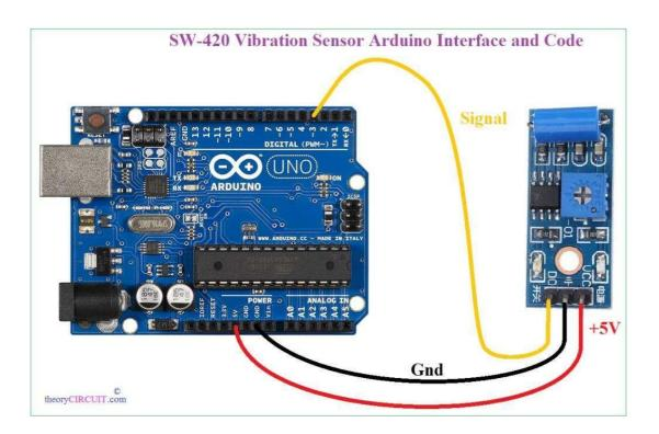
Connect Vcc pin of sensor board to 5V pin of Arduino board, connect Gnd pin to Gnd pin of Arduino, Connect DO output signal pin of sensor board to Arduino digital pin D3. Do some calibration and adjust the sensitivity threshold, then upload the following sketch to Arduino board.
