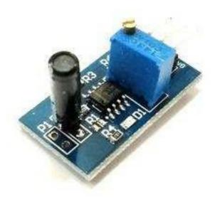
This module features an adjustable potentiometer, a vibration sensor, and a LM393 comparator chip to give an adjustable digital output based on the amount of vibration. The potentiometer can be adjusted to both increase and decrease the sensitivity to the desired amount. The module outputs a logic level high (VCC) when it is triggered and a low (GND) when it isn't. Additionally there is an onboard LED that turns on when the module is triggered.
