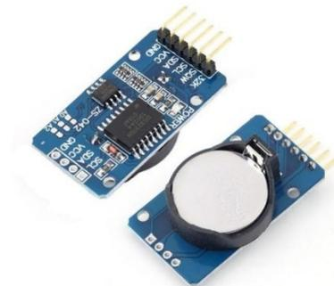
**Gambar 2. 8 Real-Time Clock (RTC)**
