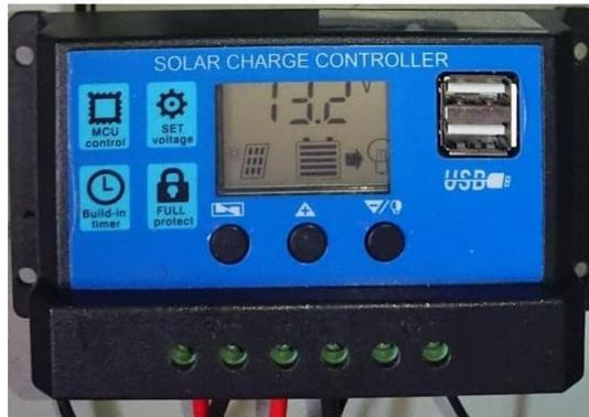
**Gambar 2. 6 Solar Charge Controller**
