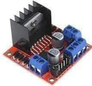
Gambar 2.7 Driver Motor L298N
