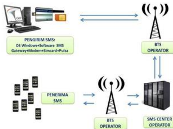
Gambar 2.2 Cara Kerja SMS Gateway
