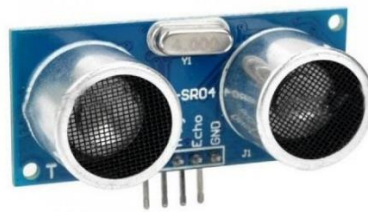
Gambar 2.3 Sensor Ultrasonik HC-SR04 (sumber: www.eu.diigit.com )
