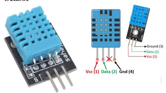
The DHT11 is a commonly used Temperature and humidity sensor that comes with a dedicated NTC to measure temperature and an 8-bit microcontroller to output the values of temperature and humidity as serial data.
