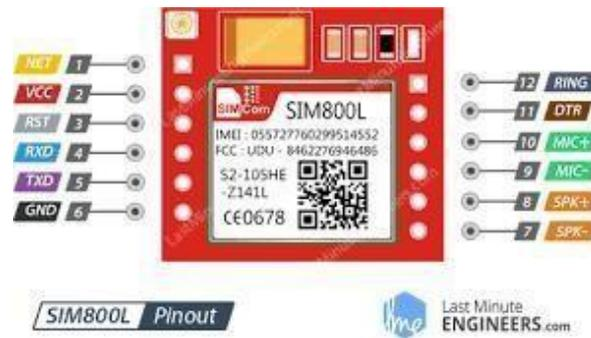
**Gambar 2.8 Pinout SIM800L**
