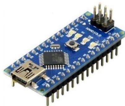
**Gambar 2.5 Arduino Nano ATmega 328P**
