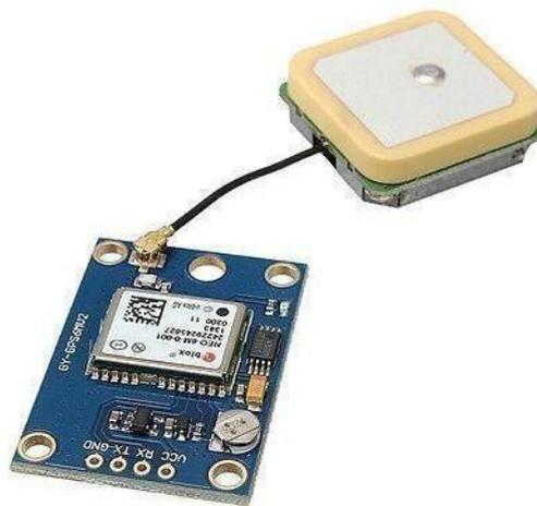
**Gambar 2.3 Modul GPS NEO-6M**
