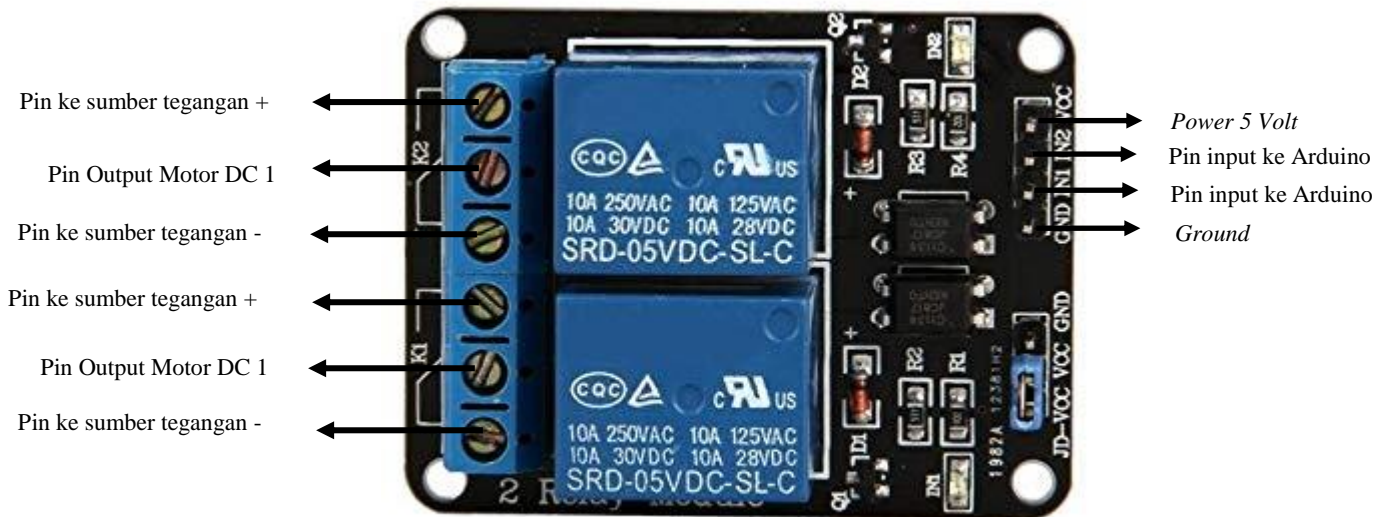
Gambar 3. 5 Perancangan Rangkaian Driver relay
