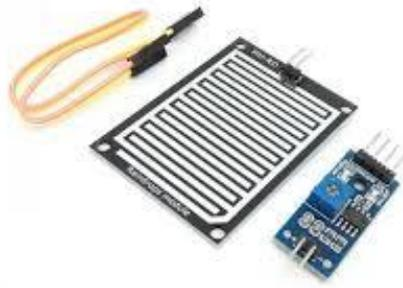
**Gambar 2.2 Sensor Hujan (Rain Sensor Arduino)**
