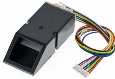
**Gambar 2.6 Sensor Fingerprint**
