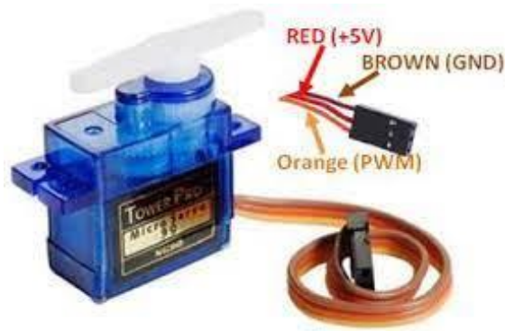
Gambar 2. 6 Motor Servo
