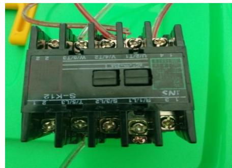
**Gambar 2.11 Kontaktor Magnet (Electric)**
