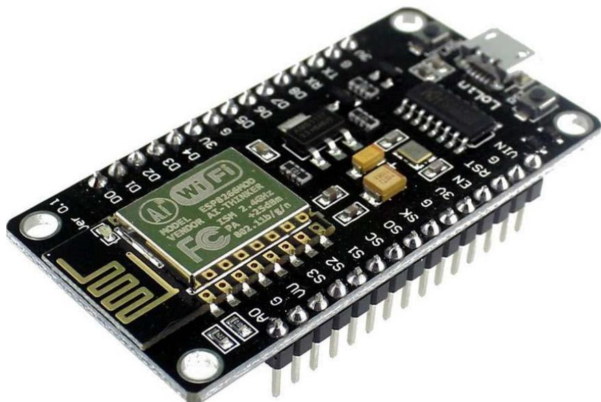
The ESP8266 is the name of a micro controller designed by Espressif Systems. The ESP8266 itself is a self-contained WiFi networking solution offering as a bridge from existing micro controller to WiFi and is also capable of running self-contained applications.
