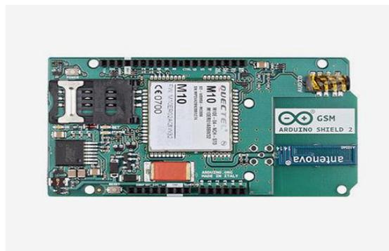
**Gambar 2.16 *Internet Shield (GSM)***
