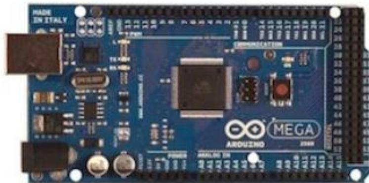
**Gambar 2.18 Arduino Mega 2560**
