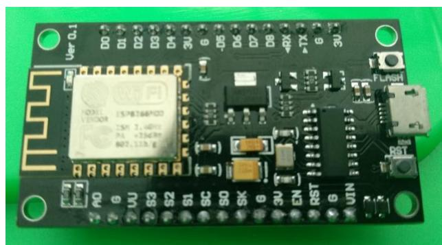
Gambar 2.1 NodeMCU ESP8266
