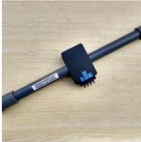
**Gambar 2. 6 Sensor Viscosity**
