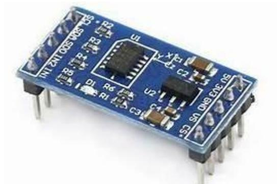
Gambar 2 Sensor accelerometer ADXL345
