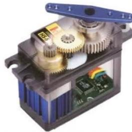
Gambar 2. 4 Sistem Mekanik Motor Servo
