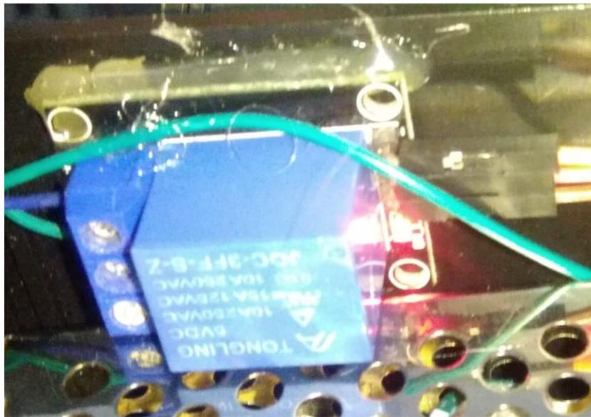
**Gambar 4.3 LED Indikator Driver Relay**
