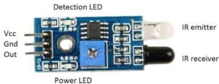
Gambar 2 4 Sensor Infrared (sumber: https://www.edukasiaelektronika.com )
