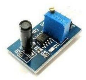
This module features an adjustable potentiometer, a vibration sensor, and a LM393 comparator chip to give an adjustable digital output based on the amount of vibration. The potentiometer can be adjusted to both increase and decrease the sensitivity to the desired amount. The module outputs a logic level high (VCC) when it is triggered and a low (GND) when it isn't. Additionally there is an onboard LED that turns on when the module is triggered.
