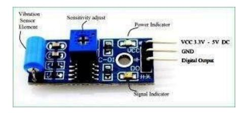
This sensor module produce logic states depends on vibration and external force applied on it. When there is no vibration this module gives logic LOW output. When it feels vibration then output of this module goes to logic HIGH. The working bias of this circuit is between 3.3V to 5V DC.
