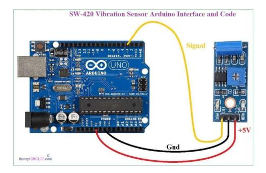
Connect Vcc pin of sensor board to 5V pin of Arduino board, connect Gnd pin to Gnd pin of Arduino, Connect DO output signal pin of sensor board to Arduino digital pin D3. Do some calibration and adjust the sensitivity threshold, then
