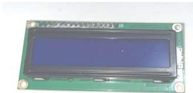
*Gambar 2. 8 LCD 16x2*
