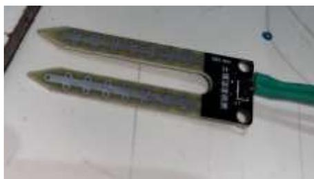
Gambar 2. 3 Sensor Soil Moisture
