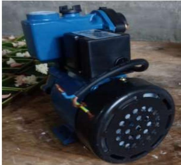
*Gambar 2. 5 Pompa Air*
