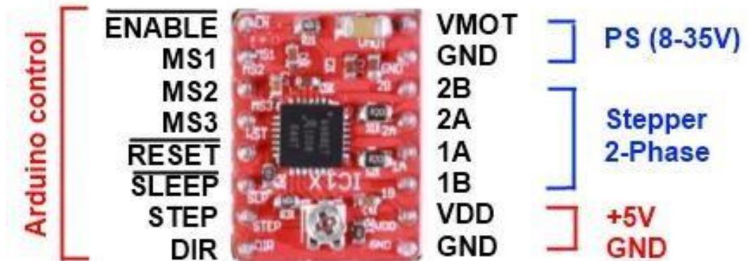
**Gambar 2. 15 Diagram Fungsi Driver Motor**
