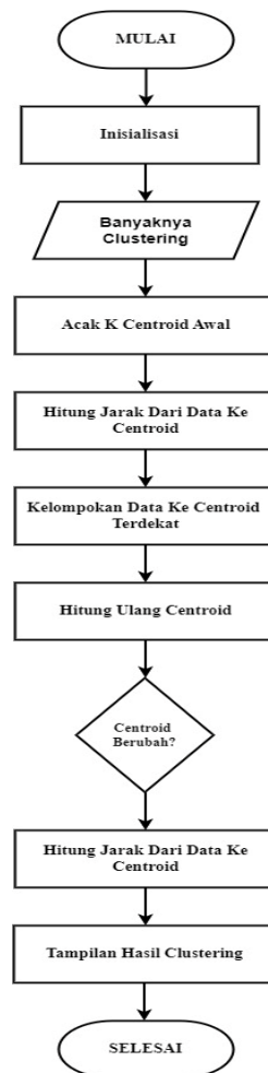
Gambar 2. 2 Flowchart Proses Algoritma K-Means
