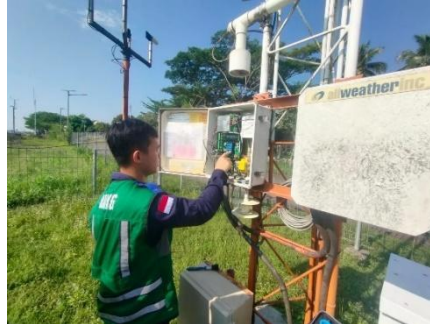
Gambar 21. Pengecekan Automatic Weather Station (AWS)
