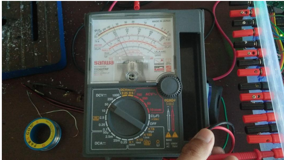
Gambar 4.3. Pengukuran Power Supply 12V
