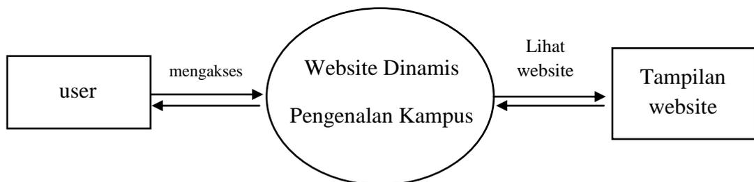
**Gambar 3.3 Rancangan *Data Flow Diagram* (DFD) Level 0**
