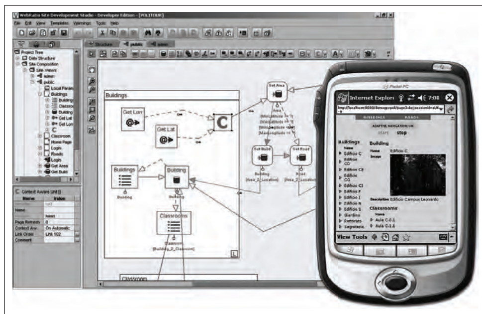
Figure 9. The WebRatio CASE tool showing the hypertext model of the buildings page with respective adaptivity actions and the generated PoliTour application running on a PDA
