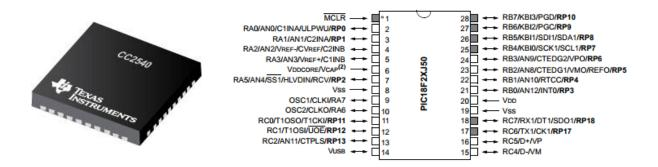
Figure 8.25. Left: the CC2540 integrated Bluetooth chip from Texas instruments. Right: the PIC18F26J50 schematic.
