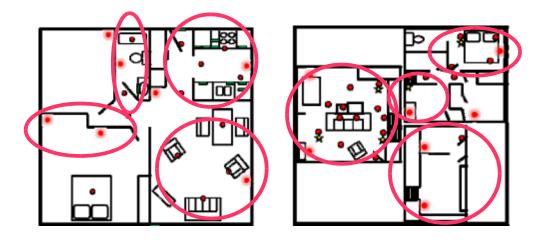
Figure 7.14. Bosch and Cairo test-bed smart environments used by Cook (2012). The encircled sensor groups are the opportunities for sensor cluster-tree grouping. The small red dots are the smart home sensors.
