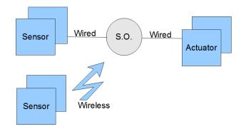
Figure 7.8. A smart object with its peripheral sensors and actuators.
