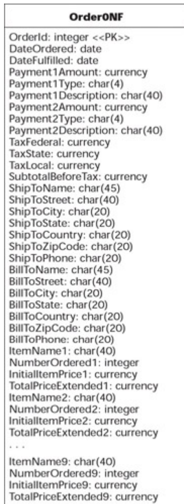
Figure 4.1: An initial data schema for order (UML notation).
