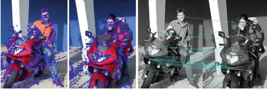
Fig. 11 Left Features identified and Right Correspondences marked for a pair of images
