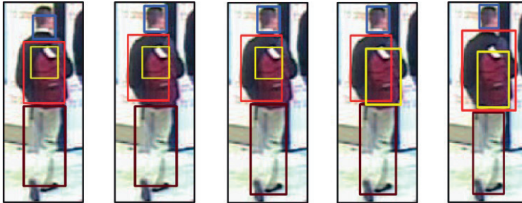
Figure 8.12 Illustration of the iterative hidden state estimation for a sample image (and matching attribute profile). Far left: initial estimate of the partition state \mathbf{Z} . Far right: final converged estimate of the partition state, leading to an increased match score. Not pictured: corresponding estimates of the hidden mixture states \{\boldsymbol{\pi}_i\}_{i=1}^N , which determine the conditional probability of the observations within each component.
