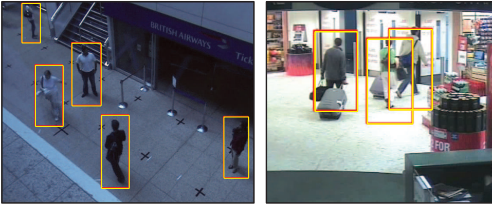
Figure 8.2 Detections of moving persons in sample video frames from two different airport environments. The first frame is from the Performance Evaluation of Tracking and Surveillance (PETS) dataset [7], and the second is from the i-LIDS Multiple Camera Tracking Dataset [8].
