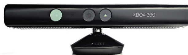
5.13 The Kinect camera has a built-in RGB camera, infrared light, and depth sensor,
