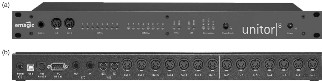
Figure 5.24 Front and back panels of the Emagic Unitor 8 interface, showing USB port, RS-422 port, RS-232 port, LTC and VTC ports and multiple MIDI ports
