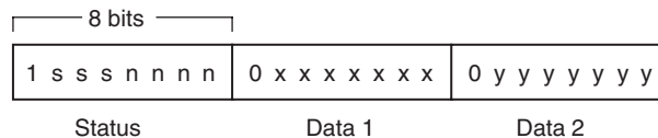
Figure 4.6 General format of a MIDI message. The ‘sss’ bits are used to define the message type, the ‘nnnn’ bits define the channel number, whilst the ‘xxxxxx’ and ‘yyyyyy’ bits carry the message data. See text for details
