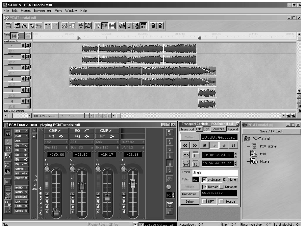
Figure 7.9 SADiE editor displays, showing mixer, playlist, transport controls and project elements
