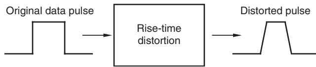
Figure 5.23 The edges of a square pulse subjected to rise-time distortion
