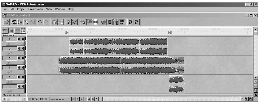
Figure 3.15 Example from SADIE editing system, showing audio clips assigned to different tracks on a virtual tape, against a timeline
