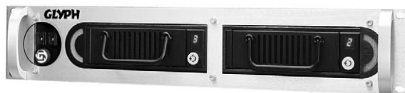
Figure 5.6 A typical removable disk drive system allowing multiple drives to be inserted or removed from the chassis at will (Courtesy of Glyph Technologies, Inc.)
