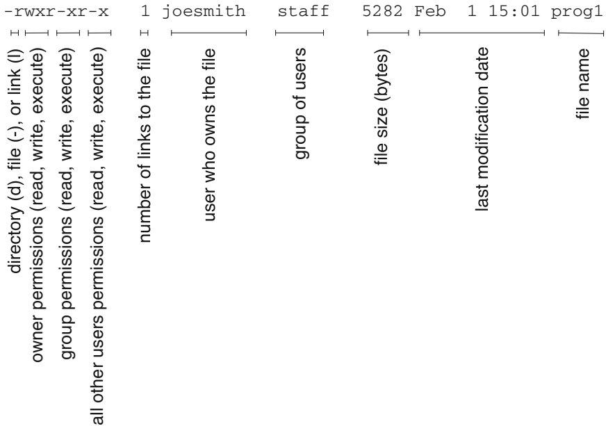
Fig. 3.5 Display format for the ls -l command for an executable file named prog1 , owned by user joesmith . See text for more details
