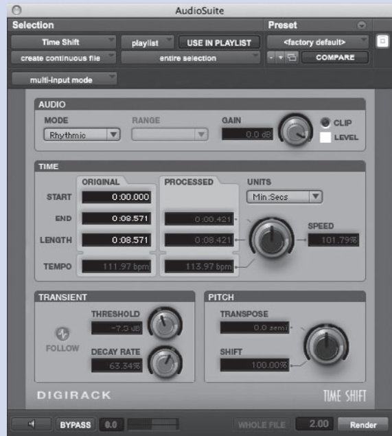
FIGURE 12.7 The Time Shift AudioSuite plug-in is the place to go in Pro Tools for offline (rendered) time-stretching. Pitch-shifting abilities are also integrated into the plug-in, but both the pitch and time aspects can be treated separately.
