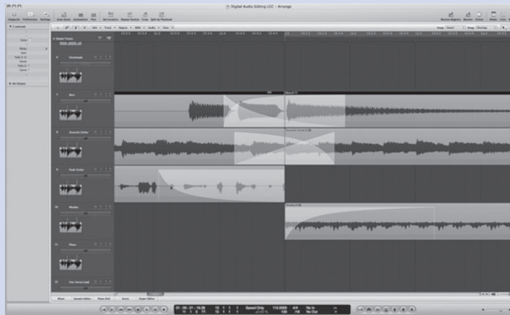
FIGURE 4.8 There are many different options for fades and cross-fades in Logic, including equal power and equal gain options and fully variable logarithmic and exponential curves.
