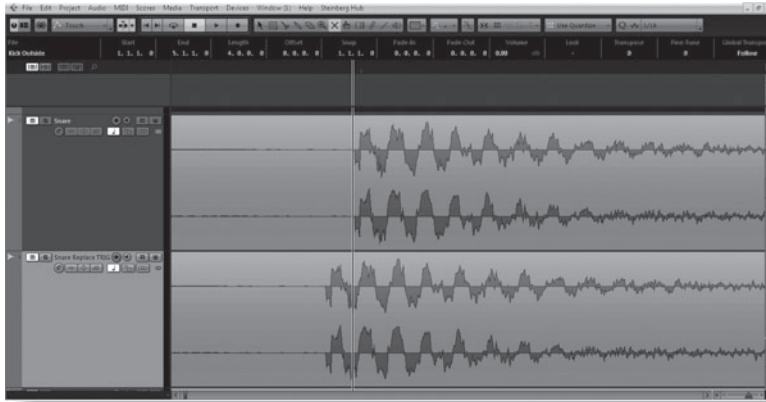
FIGURE 11.2 If the detection process means an unacceptable latency, then you can always offset the track used to trigger the detection. Here we can see the original snare drum track (at the top) and the offset copy, which is moved a few milliseconds earlier to counteract the delay in the detection process.
