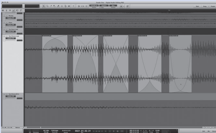
FIGURE 4.10 While there is not a huge number of options for fades and cross-fades in Studio One, it is exceptionally easy to create and edit the curves by clicking and dragging left to right to change the length, and up and down to change the shape.
