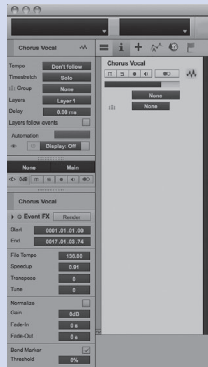
FIGURE 12.8 The Inspector Panel in Studio One has a number of different options for time-stretching algorithms as well as a place to define the original tempo of the material (if known) and a “Speedup” factor that can stretch or compress the audio by a fixed percentage in addition to any change that may have been affected automatically by following the tempo of the song.
