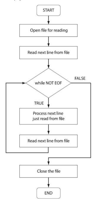
Figure 10-2: Flow chart illustrating the algorithm to process a file of records
