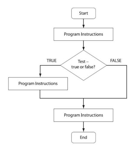
Figure 7-2 General-purpose Flow Chart showing an IF structure
