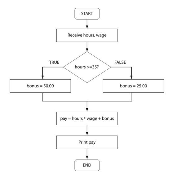
Figure 7-5: Flow Chart showing the algorithm for wage4.php
