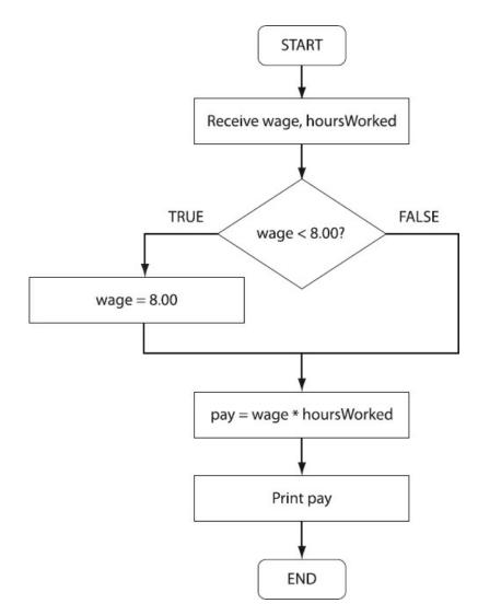
Figure 7-4: Flow Chart showing the algorithm for wage3.php
