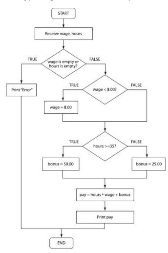
Figure 8.2 Flow Chart showing the algorithm for wage7.php
