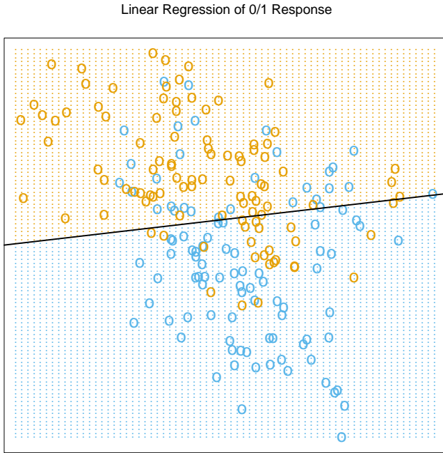
FIGURE 2.1. A classification example in two dimensions. The classes are coded as a binary variable (BLUE = 0, ORANGE = 1), and then fit by linear regression. The line is the decision boundary defined by x^T \hat{\beta} = 0.5 . The orange shaded region denotes that part of input space classified as ORANGE, while the blue region is classified as BLUE.
