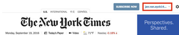
Fig. 3 The email address of a logged-in New York Times user is displayed on the top banner of the website (highlighted in red). Because the New York Times does not deliver their webpage over an encrypted connection (as of September 2016), an eavesdropper can use the email address to assign a real-world identity to a pseudonymous web browser
