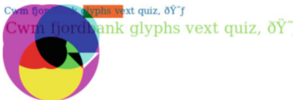
Fig. 1 The image, invisible to the user, that is drawn on the web page by one of the canvas fingerprinting scripts that we detected. The image is converted to a string of data, constituting the fingerprint
