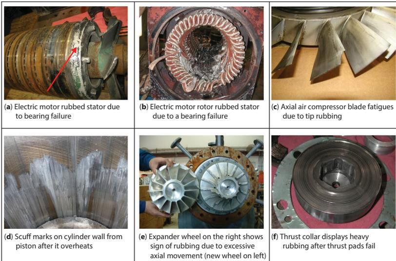
**Figure 3.6** Failure resulting from rubbing examples.
