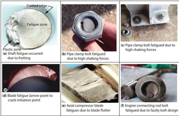
Figure 3.3 Fatigue failures.
