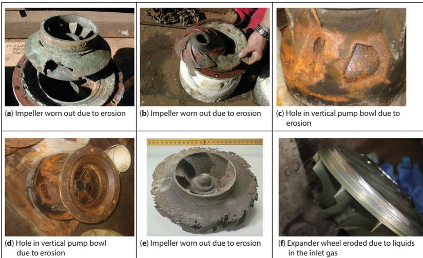
**Figure 3.2** Examples of erosive wear failures.
