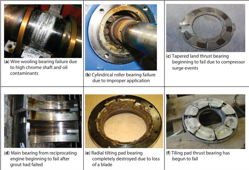
**Figure 3.5** Bearing failure examples.
