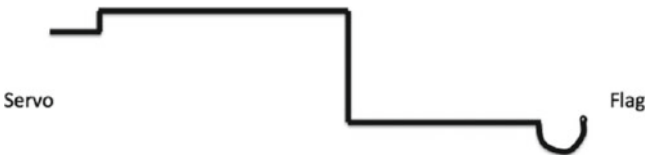
Figure 14-14. Forming the servo rod/cable
