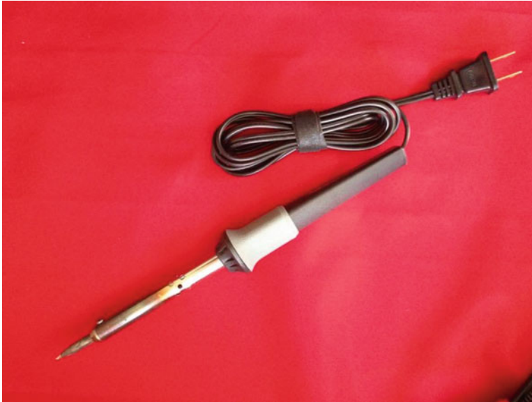
Figure 8-2. Entry-level soldering iron
