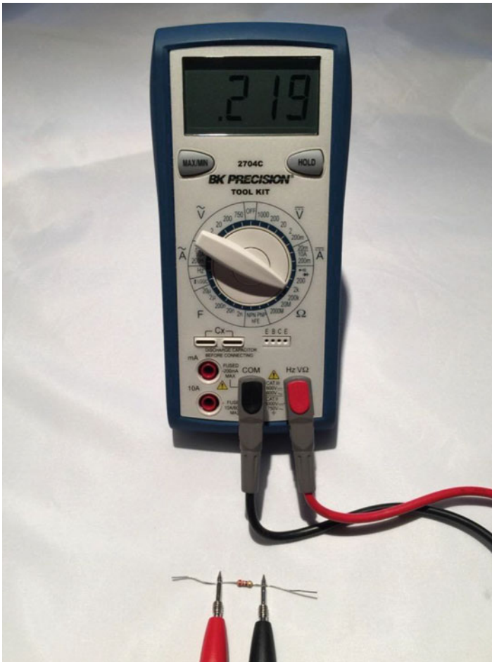
Figure 8-11. Measuring resistance of a resistor
