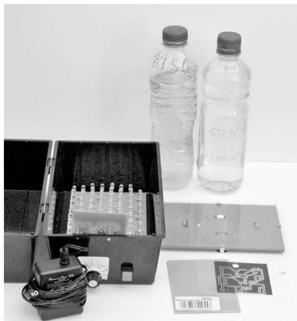
FIGURE 7.9 A photo-etching kit.
