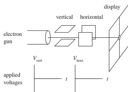
When no voltages are applied to the horizontal and vertical plates, the electron beam is focused at the center of the scope's display.
