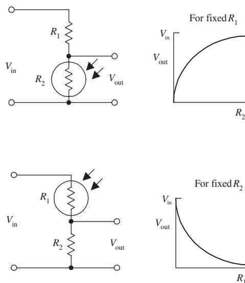
These circuits resemble the voltage-divider circuit described in Chap. 3. As before, the output voltage is given by
