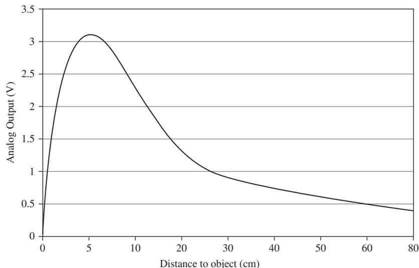
FIGURE 6.14 Output against distance for a Sharp GP2Y0A21YK.
