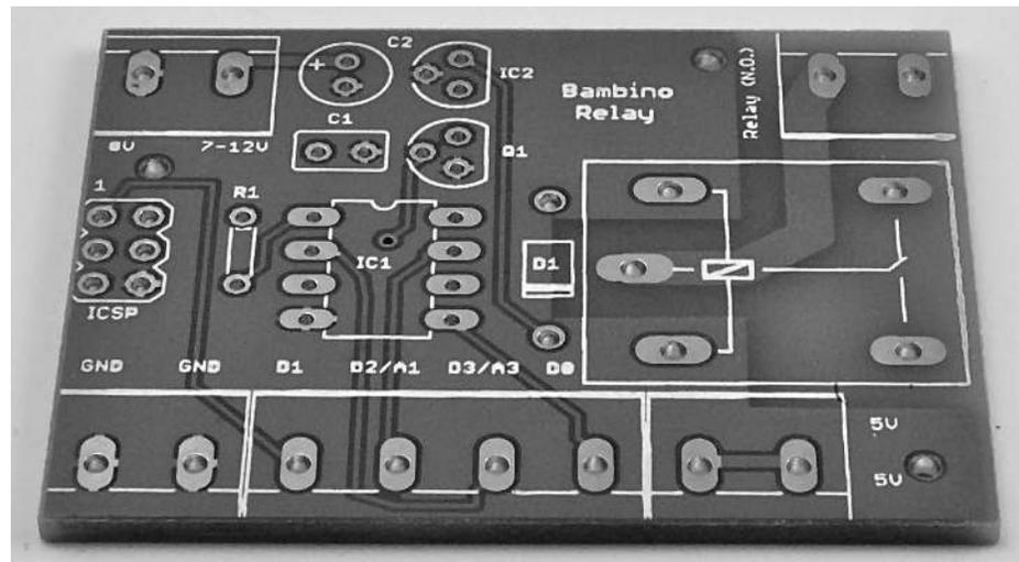
FIGURE 7.11 A PCB created by a PCB services.
