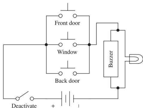
Here’s a simple home security alarm that’s triggered into action (buzzer and light go on) when one of the normally open switches is closed. Magnetic reed switches work particularly well in such applications.
