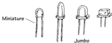
These LEDs are inexpensive and durable devices that typically are used as indicator lights. Common colors include green (~565 nm), yellow (~585 nm), orange (~615 nm), and red (~650 nm). Maximum forward voltages are about 1.8 V, with typical operating currents from 10 to 30 mA.
