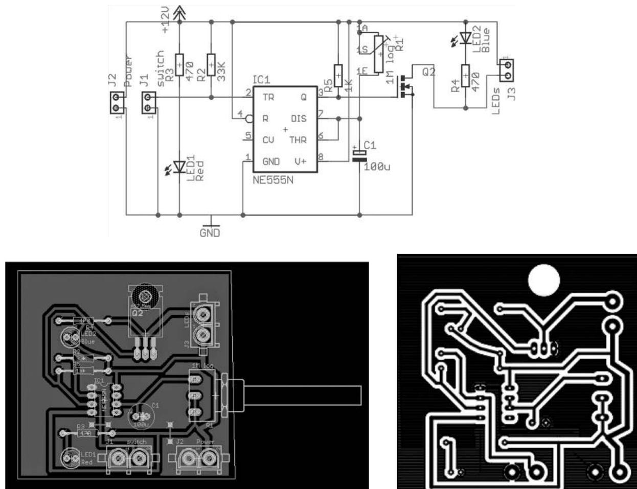
FIGURE 7.8 EAGLE PCB, schematic and copper layer.
