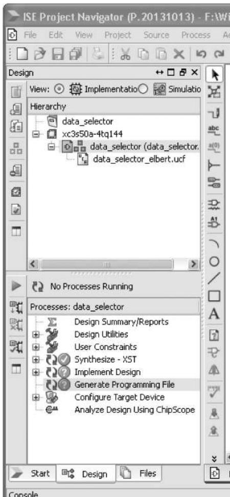
FIGURE 14.17 Generating the programming file.
