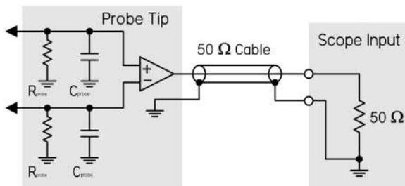
34 MHz). The 10X probe introduces about ten times less capacitance. Bandwidth differences also apply to 100X and 1000X probes.
