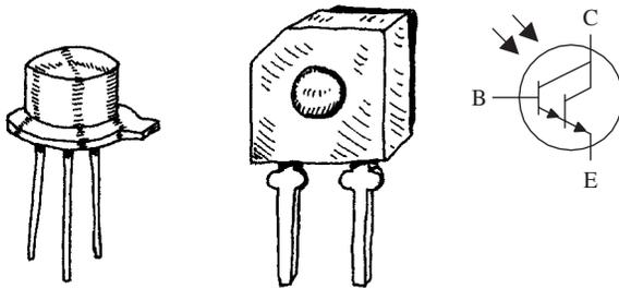
This is similar to a conventional bipolar Darlington transistor but is light-sensitive. Photodarlingtons are much more sensitive to light than ordinary phototransistors, but they tend to have slower response times. These devices may or may not come with a base lead.
