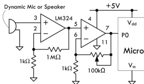
This circuit uses an LM324 comparator IC connected to a dynamic microphone or speaker. When a specific sound level is reached—set by pot, the output suddenly changes, supplying a HIGH to the microcontroller's input.
