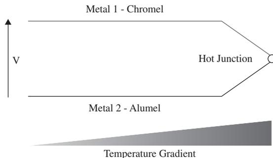
FIGURE 6.7 Thermocouples.
