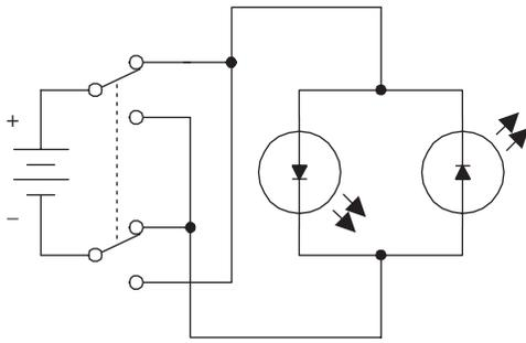
A DPDT switch, shown here, can be used to reverse the direction of current flow. When the switch is thrown up, current will flow through the left light-emitting diode (LED). When the switch is thrown down, current will flow through the right LED. (LEDs only allow current to flow in one direction.)
