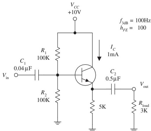
Fortunately, you can make an approximation and simply let  $R_1 = R_2$ . This approximation “forgets” the 0.6-V drop but usually isn’t too dramatic. The actual sizes of  $R_2$  and  $R_1$  should be such that their parallel resistance is less than or equal to one-tenth the dc (quiescent) input resistance at the base (this prevents the voltage divider’s output voltage from lowering under loading conditions):
