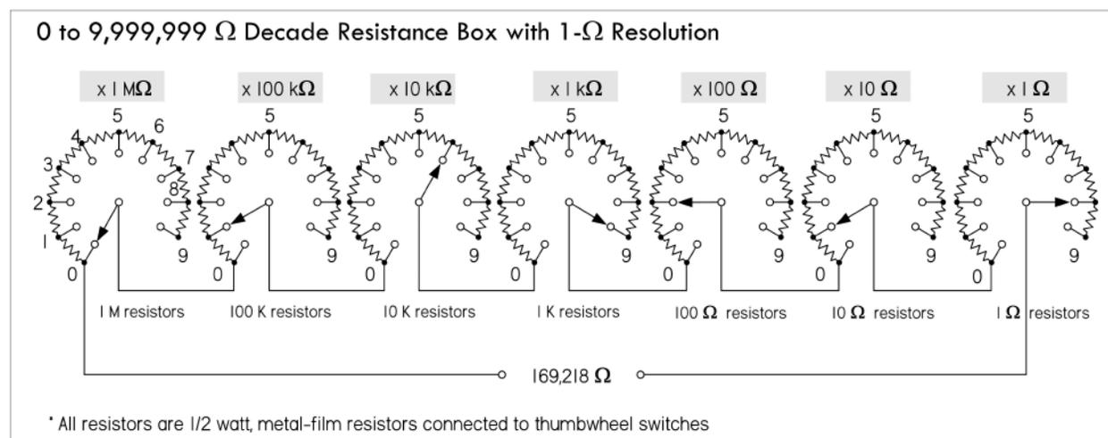
FIGURE 7.67 Resistor decade box made using thumbwheel switches.
