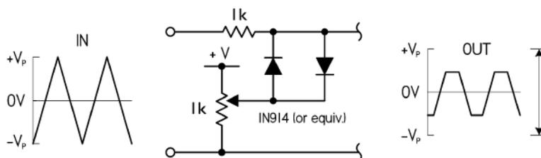
The adjustable attenuator is similar to the last circuit, but the additional opposing diode allows for clipping on both positive and negative swings. You can use separate potentiometers if you want separate positive and negative clipping level control. +V should be a volt or so higher than the peak input voltage.
