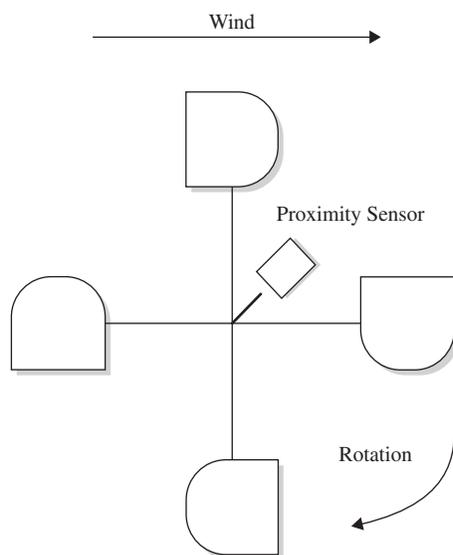
**FIGURE 6.22** A cup anemometer.
