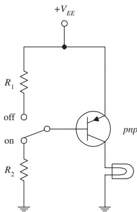
In the *pnp* circuit, everything is reversed; current must leave the base in order for a collector current to flow.
