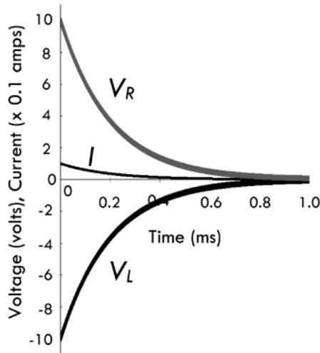
The graph shown in the figure is for a circuit with  $R = 100 \Omega$  and  $L = 20 \text{ mH}$ .
