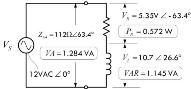
Sinusoidal Waveforms within Series RL Circuit
