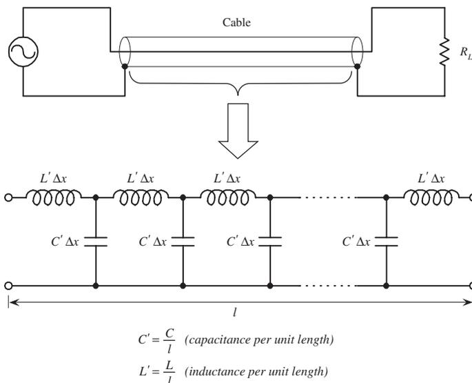
The impedance of a cable can be modeled by treating it as a network of inductors and capacitors.
