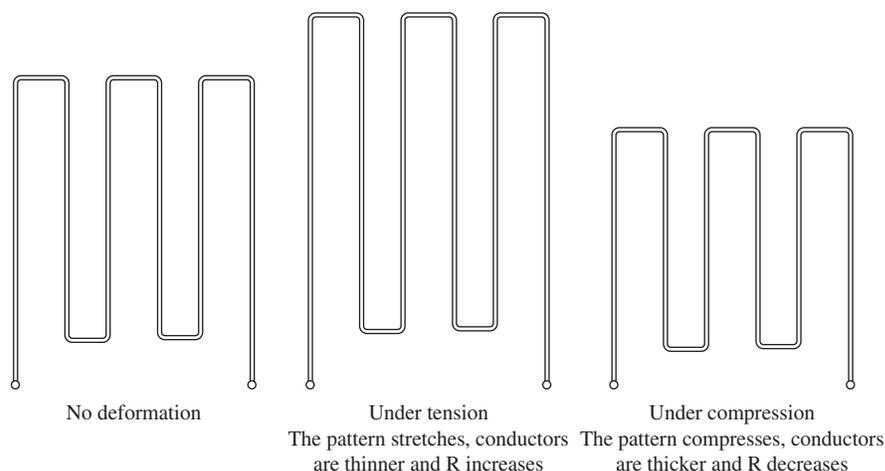
**FIGURE 6.23 Strain gauge.**
