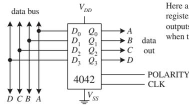
Here a 4042 is used as a 4-bit data register. Data on bus appears at outputs. Data is latched (saved) when the clock switches states.
