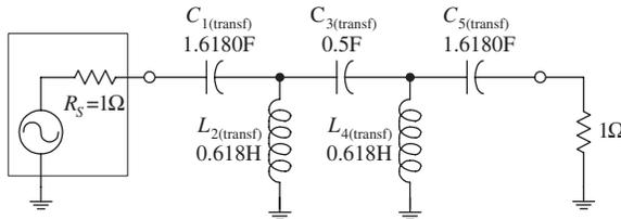
Impedance and frequency scale high-pass filter to get final circuit
