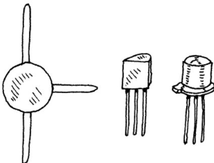
These transistors are used for small signals that run at high frequencies for high-speed switching applications. The base region is very thin, and the actual chip is very small. They are used in HF, VHF, UHF, CATV, and MATV amplifier and oscillator applications. They have a maximum frequency rating of around 2000 MHz and maximum  $I_C$  currents from 10 to 600 mA. They come in both *npn* and *pnp* forms.
