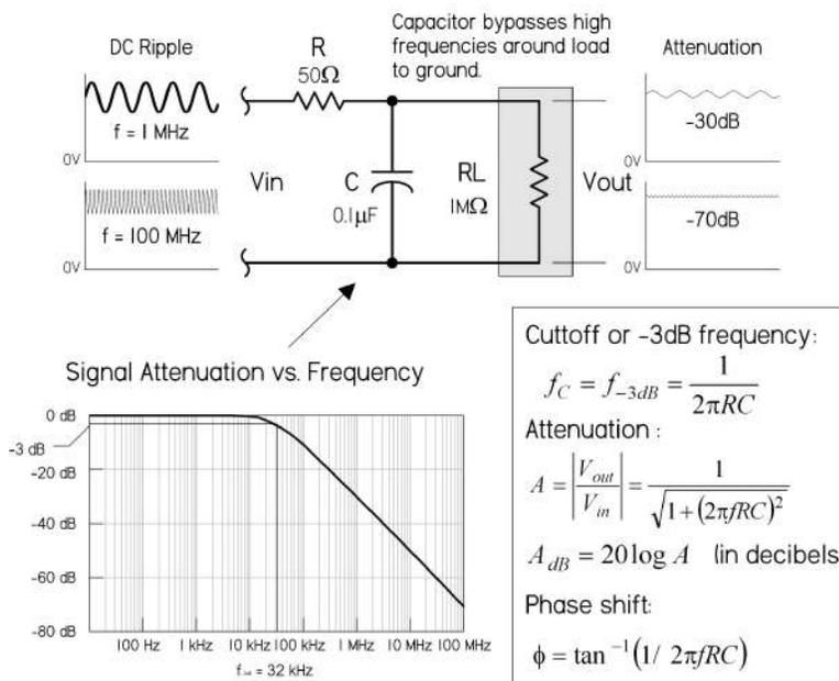
In this circuit, the RC section acts like a low-pass filter, which attenuates high frequencies from reaching the load or circuit element.
