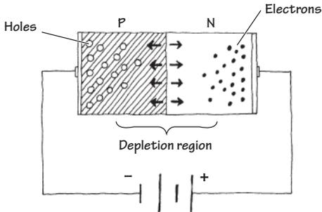
When a diode is connected to a battery, as shown here, holes in the *n* side are forced to the left, while electrons in the *p* side are forced to the right. This results in an empty zone around the *p-n* junction that is free of charge carriers, better known as the *depletion region*. This depletion region has an insulative quality that prevents current from flowing through the diode. When a diode is arranged in this way, it is said to be *reverse-biased*.
