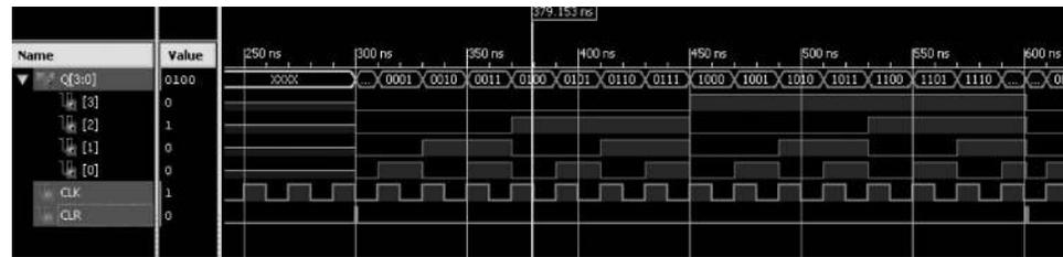
FIGURE 14.33 Simulation results for the counter.
