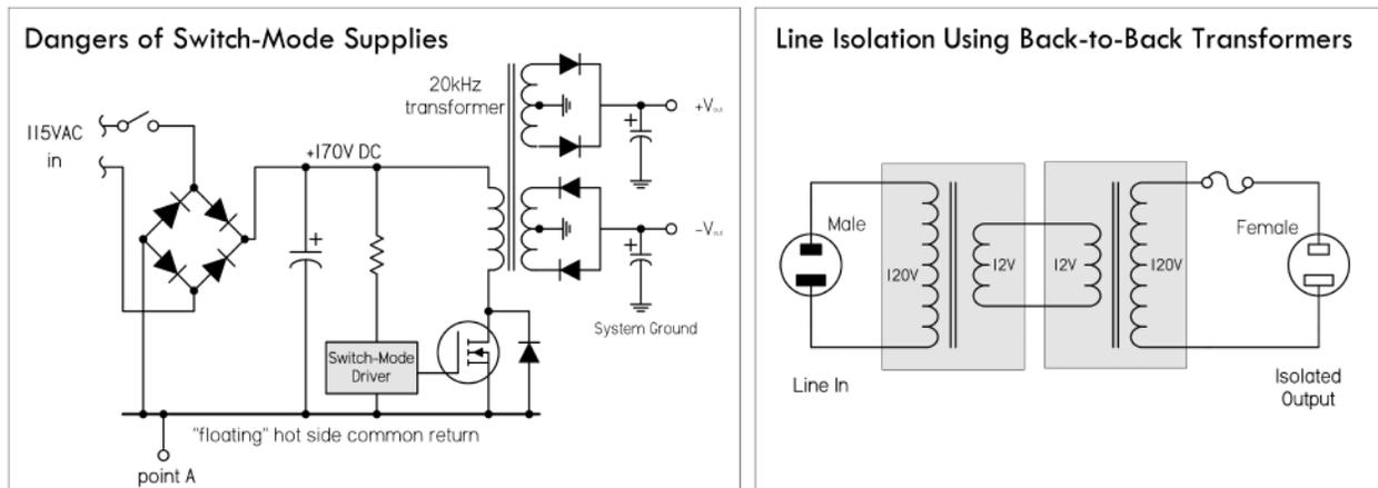
**FIGURE 7.64** The illustration on the left shows how a switch-mode supply can be dangerous. Without the use of an isolation transformer, a ground lead of a scope connected to point A will blow out one of the bridge diodes, while vaporizing the scope probe tip. The illustration on the right shows how to construct a simple isolation transformer using two standard 120-V/12-V transformers, back to back.
