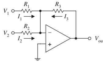
Since you know that  $V_+$  is grounded (0 V), and since you have negative feedback in the circuit, you can say that  $V_+ = V_- = 0V$  (rule 4). Now that you know  $V_-$ , solve for  $I_1$ ,  $I_2$ , and  $I_3$  in order to come up with an expression relating  $V_{out}$  with  $V_1$  and  $V_2$ . The currents are found by applying Ohm's law:
