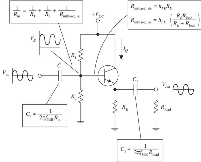
To design a common-collector amplifier used to power a 3-kΩ load, which has a supply voltage  $V_{CC} = +10\text{ V}$ , a transistor  $h_{FE}$  of 100, and a desired  $f_{3dB}$  point of 100 Hz, you
