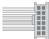
IDC connectors are often found in computers. The plug is attached to ribbon cable using v-shaped teeth that are squeezed into the cable insulation to make a solderless contact.
