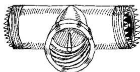
T-connectors consist of two plug ends and one central jack end. They are used when a connection must be made somewhere along a coaxial cable.
