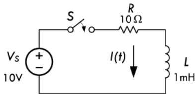
$$I(t) = \begin{cases} 0 & t < 0 \text{ (before S closed)} \\ 0 & t = 0 \text{ (S just closed)} \\ (V_S / R)(1 - e^{-(R/L)t}) & t > 0 \text{ (after S closed)} \\ V_S / R & t \rightarrow \infty \text{ (steady state)} \end{cases}$$
