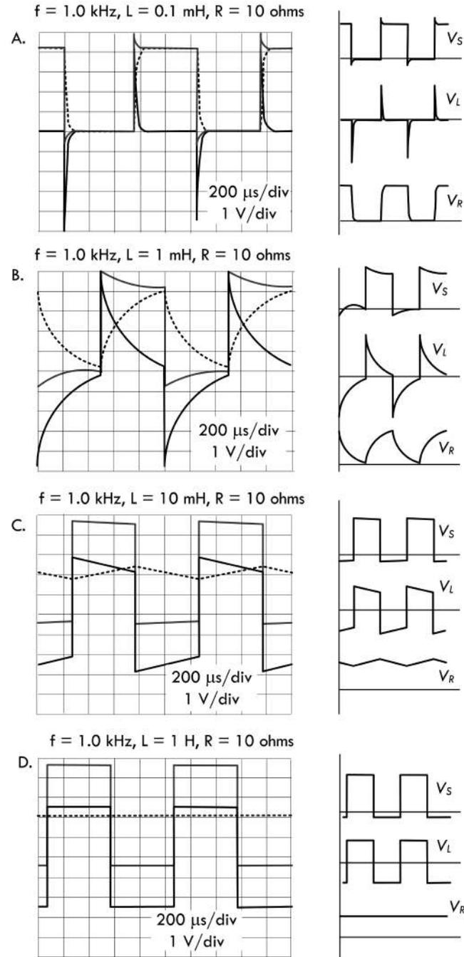
Inductance, be it intended or not, can have a major influence on signals. For example, the output signals across the inductor and resistor in the RL circuit to the left become increasingly distorted as the inductance increases. With a constant 1.0-kHz, 0–5-V squarewave source, and fixed 10- $\Omega$  resistance, we increase the inductance and note the changes in the waveforms. First we note that the period of the squarewave is:
