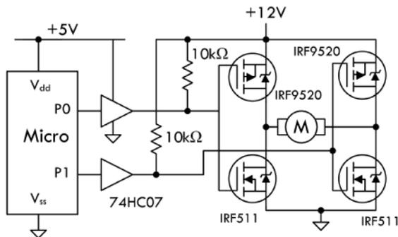
The H-bridge circuit built using MOSFETs provides forward and reverse directional control of a dc motor. The H-bridge provides built-in dynamic braking action useful for applications requiring greater control. To make motor go in one direction, P0 is set HIGH while P1 is set LOW. To switch directions, P0 is set LOW while P1 is set HIGH. Buffer stage (74HC07) could be replaced with an optoisolator to provide greater electrical isolation from motor section of circuit.
