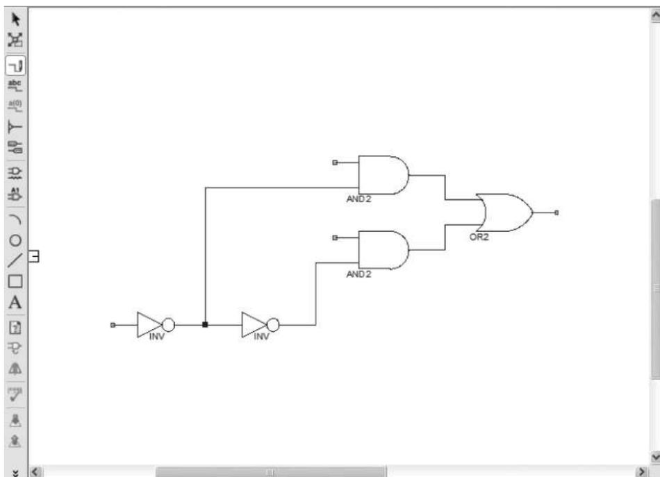
FIGURE 14.13 Connecting the symbols with wires.
