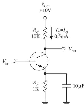
But what about  $R_E$ ? According to the circuit, there's no emitter resistor. If you use the gain formula, it would appear that  $R_E = 0 \Omega$ , making the gain infinite. However, as mentioned earlier, bipolar transistors have a transresistance (small internal resistance) in the emitter region, which is approximated by using
