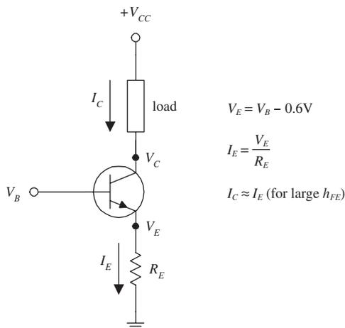
The circuit here shows how an *npn* transistor can be used to make a simple current source. By applying a small input voltage and current at the transistor's base, a larger collector/load current can be controlled. The collector/load current is related to the base voltage by
