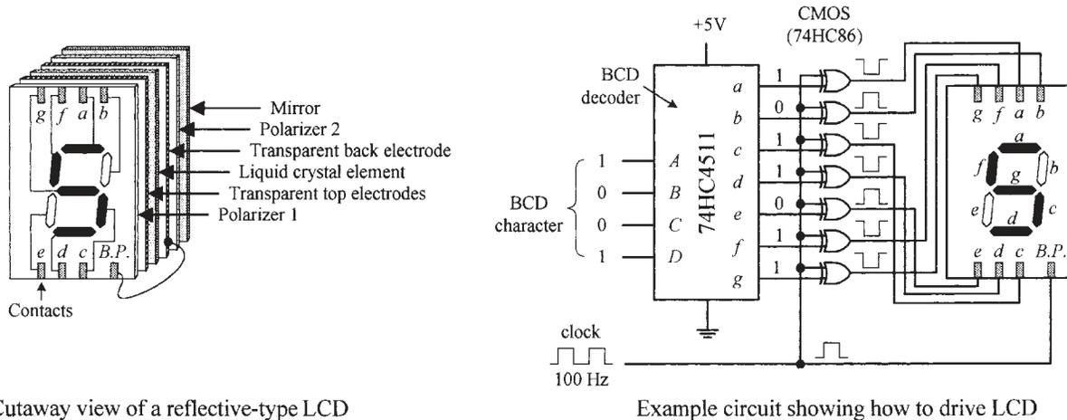
Cutaway view of a reflective-type LCD
