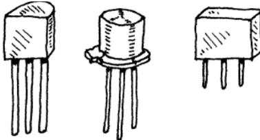
These transistors are used primarily as switches but also can be used as amplifiers. Typical  $h_{FE}$  values range from around 10 to 200, with maximum  $I_C$  ratings from around 10 to 1000 mA. They come in both *npn* and *pnp* forms. Maximum switching rates range between 10 and 2000 MHz.
