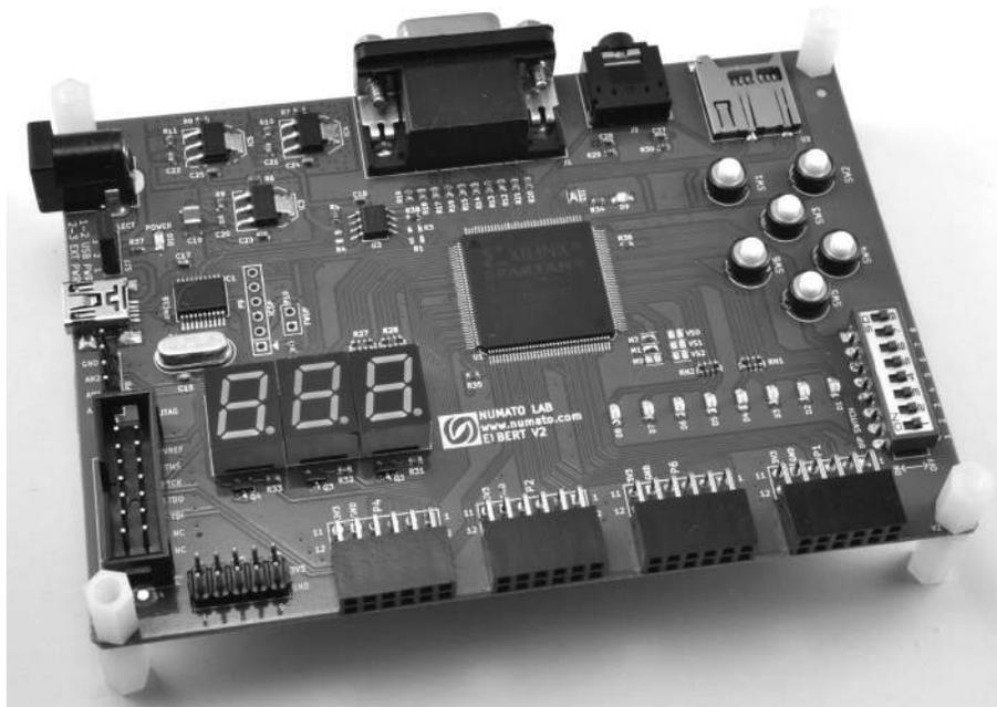
FIGURE 14.4 The Elbert 2–Spartan 3A FPGA development board.
