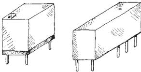
Miniature relays are similar to subminiature relays, but they are designed for greater sensitivity and lower-level currents. They are almost exclusively actuated by dc voltages but may be designed to switch ac currents. They come with excitation voltages of 5, 6, 9, and 12, and 24 V dc, with coil resistances from 50 to 3000  $\Omega$ .
