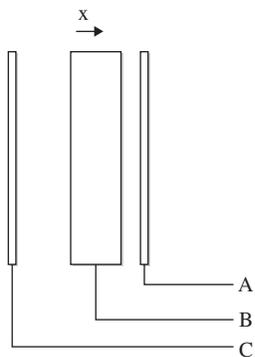
FIGURE 6.19 Measuring the offset of the mass.
