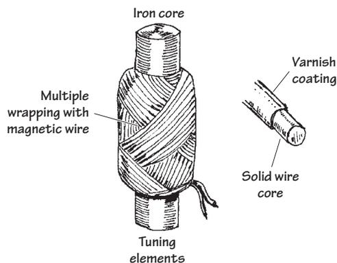
This wire is used for building coils and electromagnets or anything that requires a large number of loops, say, a tuning element in a radio receiver. It is built of solid-core wire and insulated by a varnish coating. Typical wire sizes run from 22 to 30 gauge.
