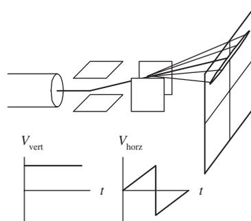
When a sawtooth voltage is applied to the horizontal plates, while no voltage is applied to the vertical plate, the electron beam traces a horizontal line from left to right. After each sawtooth, the beam jumps back to the left and repeats its left-to-right sweep.
