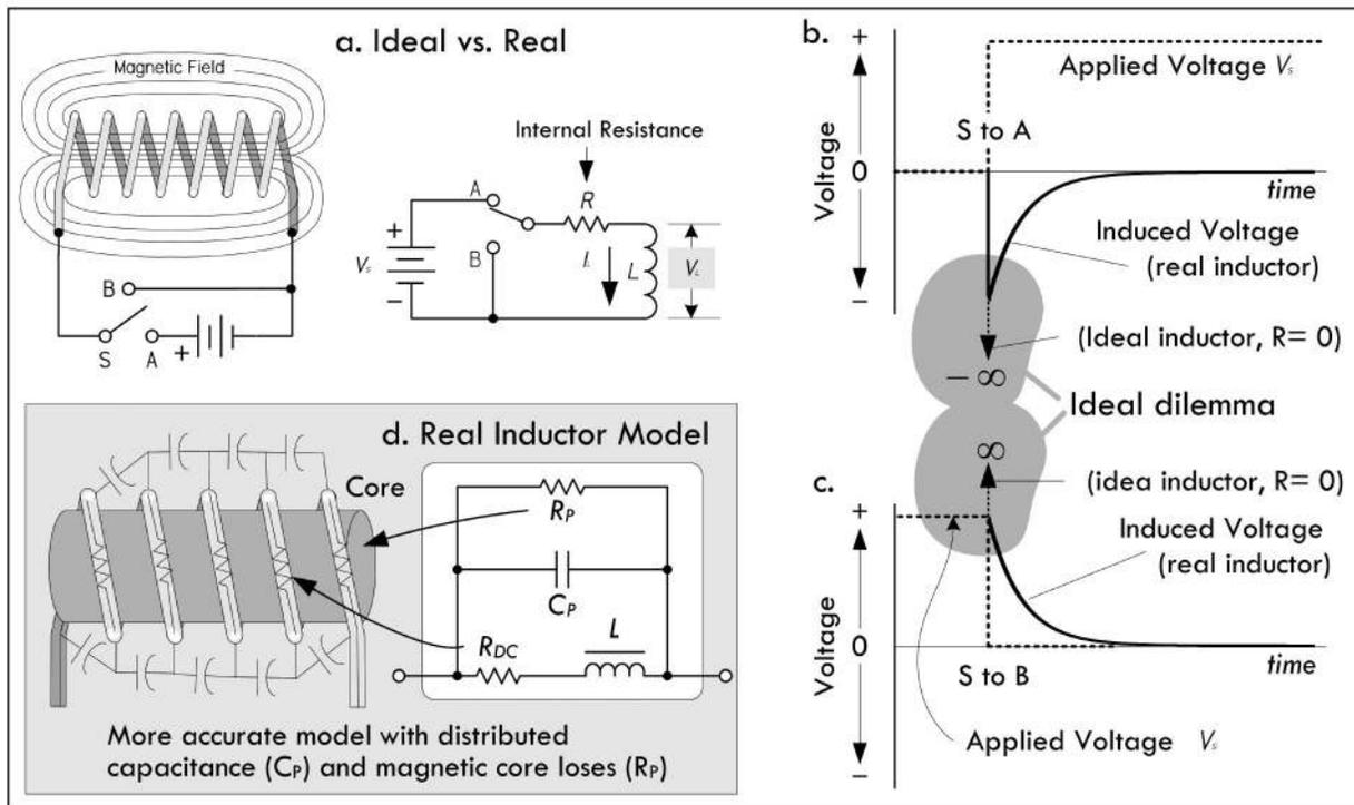
FIGURE 2.135 Real inductors never generate infinite induced voltages.
