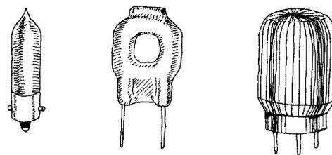
Similar to a typical incandescent lamp, these lamps provide ultrabright output light. Unlike a typical incandescent lamp, the filament is coated on the inside of a quartz bulb. Within this bulb, a halogen gas, such as bromine or iodine, is placed. These lamps are used in projector lamps, automotive headlights, strobe lights, etc.
