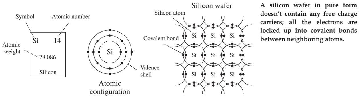
A silicon wafer in pure form doesn't contain any free charge carriers; all the electrons are locked up into covalent bonds between neighboring atoms.
