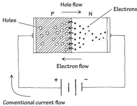
When a diode is connected to a battery, as shown here, electrons from the *n* side and holes from the *p* side are forced toward the center (*pn* interface) by the electrical field supplied by the battery. The electrons and holes combine, and current passes through the diode. When a diode is arranged in this way, it is said to be *forward-biased*.
