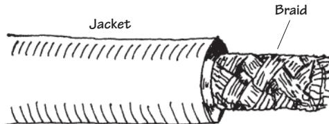
A braided wire is made up of a number of individual strands of wire braided together. Like stranded wires, these wires are better conductors than solid-core wires, and they will not break easily when flexed. Braided wires are frequently used as an electromagnetic shield in noise-reduction cables and also may act as a wire conductor within the cable (e.g., coaxial cable).
