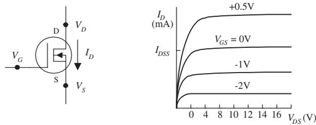
**OHMIC REGION** MOSFET is just beginning to resist. In this region, the MOSFET behaves like a variable resistor.
