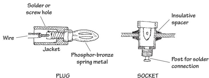
This is used for connecting single wires to electrical equipment. It is frequently used with testing equipment. The plug is made from a four-leafed spring tip that snaps into the jack.
