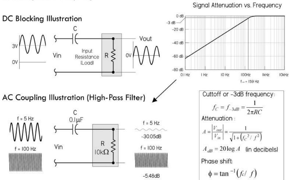
**FIGURE 3.67** *Blocking:* A capacitor is used to block or prevent dc voltages from passing from one circuit to another. To block the dc voltage, the capacitor is placed in series with the circuit element.
