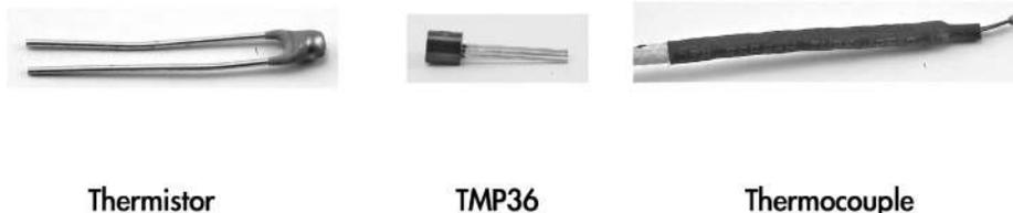
FIGURE 6.4 Temperature sensors.
