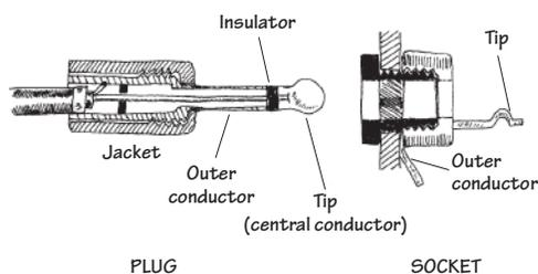
These connectors accept shielded braid, but they are larger in size. They come in two- or three-element types and have a barrel that is 1¼ in (31.8 mm) long. They are used as connectors in microphone cables and for other low-voltage, low-current applications.
