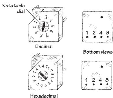
These switches are used to encode digital information. A mechanism inside the switch will “make” or “break” connections between the switch pairs according to the position of the dial on the face of the switch. These switches come in either true binary/hexadecimal and complementary binary/hexa-decimal forms. The charts below show how these switches work:
