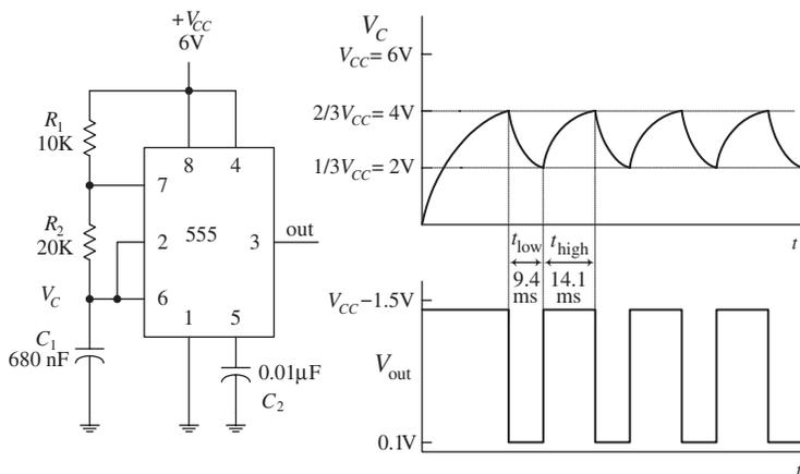
$$t_{\text{low}} = 0.693(20\text{K})(680\text{nF}) = 9.6\text{ms}$$
