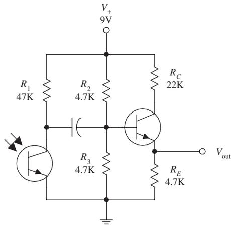
The circuit shown here illustrates how a phototransistor can be used as a modulated lightwave detector with an amplifier section (current gain amplifier).  $R_2$  and  $R_3$  are used to set the dc operating point of the power-switching transistor, and  $R_1$  is used to set the sensitivity of the phototransistor. The capacitor acts to block unwanted dc signals from entering the amplifier section.
