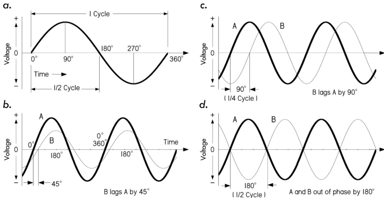
**FIGURE 2.85** (a) An ac cycle is divided into 360° that are used as a measure of time or phase. (b) When two waves of the same frequency start their cycles at slightly different times, the time difference or phase difference is measured in degrees. In this drawing, wave B starts 45° (one-eighth cycle) later than wave A, and so lags 45° behind A. (c and d) Two special cases of phase difference: In (c) the phase difference between A and B is 90°; in (d) the phase difference is 180°.
