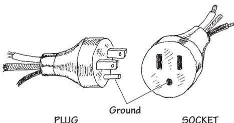
This is a typical home appliance connector. It comes in unpolarized and polarized forms. Both forms may come with or without a ground wire.
