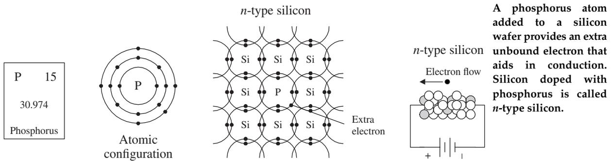
A phosphorus atom added to a silicon wafer provides an extra unbound electron that aids in conduction. Silicon doped with phosphorus is called *n-type silicon*.
