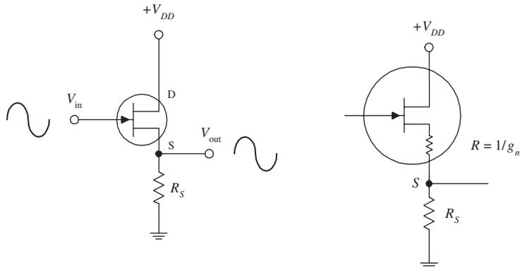
FIGURE 4.79 The JFET circuit here is called a *source follower*, which is analogous to the bipolar emitter follower; it provides current gain but not voltage gain. The amplitude of the output signal is found by applying Ohm's law:  $V_S = R_S I_D$ , where  $I_D = g_m V_{GS} = g_m (V_G - V_S)$ . Using these equations, you get
