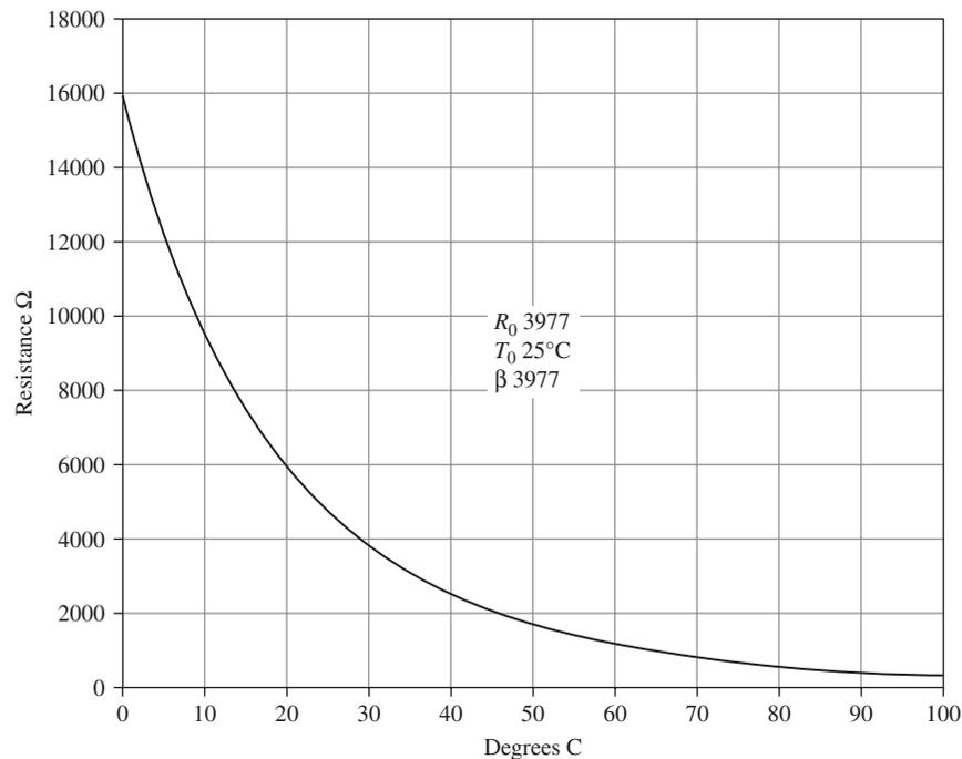
FIGURE 6.5 Resistance against temperature for an NTC thermistor.
