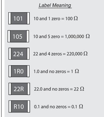
The first two digits represent significant figures; the last digit specifies the multiplier. For values under 100 Ω, the letter R is substituted for one of the significant digits and represents a decimal point.
