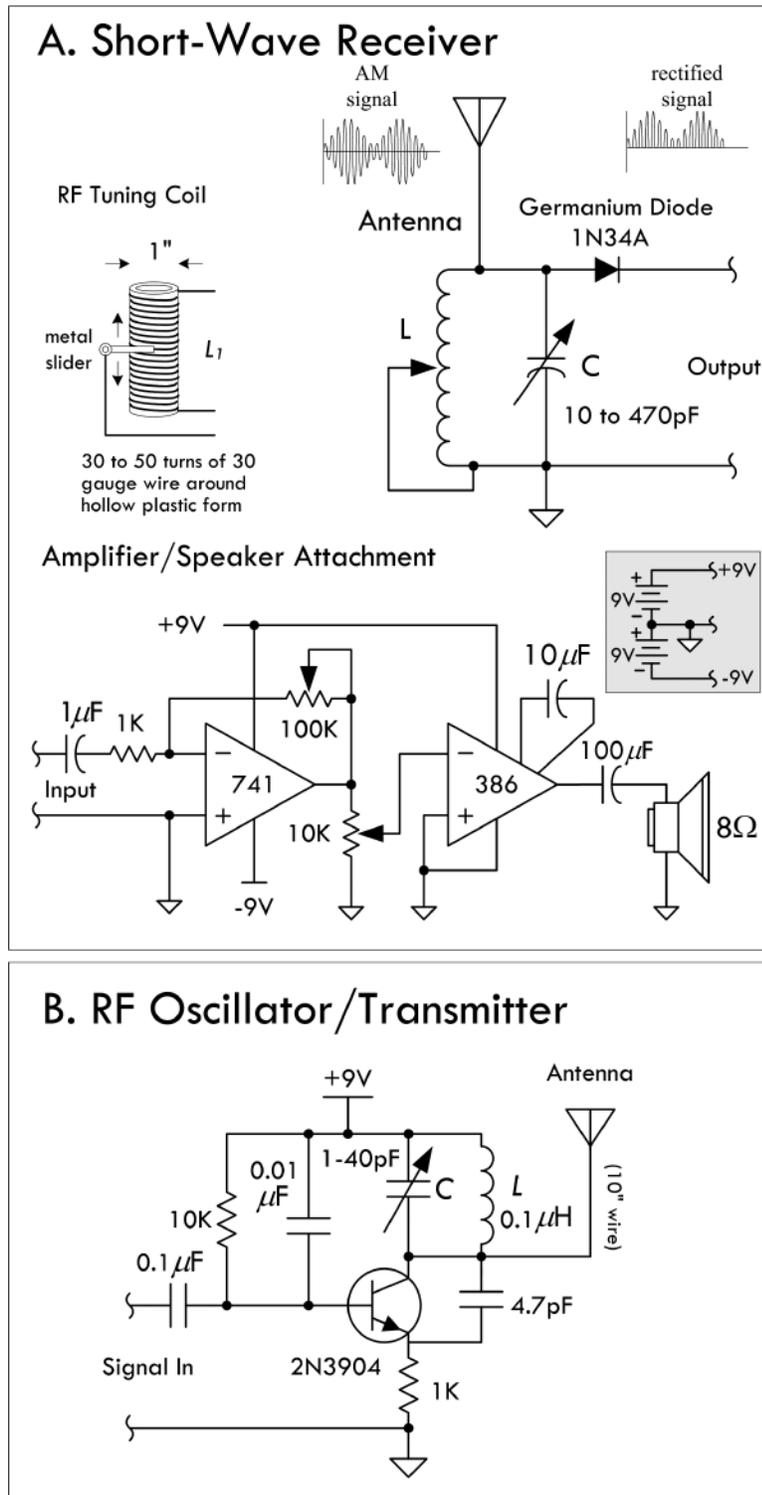
Here are a few simple radiofrequency circuits that make use of LC resonant filters to tune the circuits.
