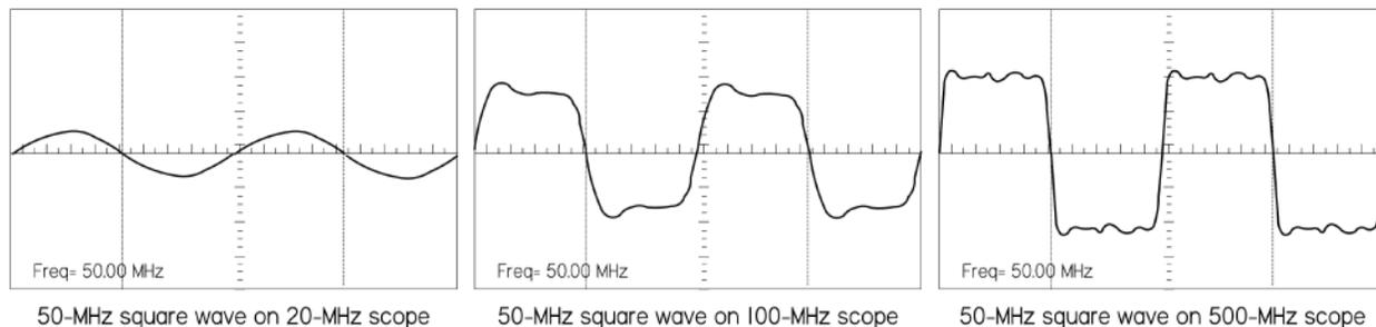
**FIGURE 7.56** Screenshots show the same 50-MHz square wave displayed on three different scopes with different bandwidths. The 500-MHz scope shows the best high-frequency detail and representation of rise times. As you move down in bandwidth, notice the increase in rise time and amplitude attenuation. The bandwidth of your scope should be at least three times the fundamental frequency of the fastest signal you expect to measure, and as much as ten times more for accurate amplitude measurements.
