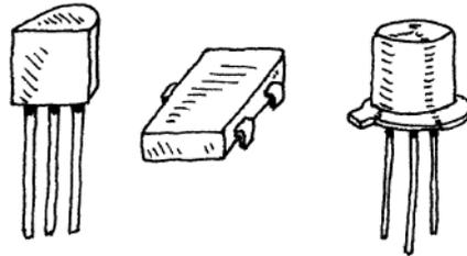
This type of transistor is used to amplify low-level signals but also can be used as a switch. Typical  $h_{FE}$  values range from 10 to 500, with maximum  $I_C$  ratings from about 80 to 600 mA. They come in both *npn* and *pnp* forms. Maximum operating frequencies range from about 1 to 300 MHz.
