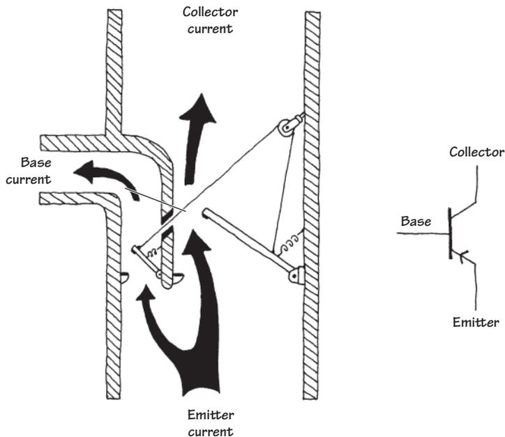
The main feature to note here is the need for a lower pressure at the base for the *pnp* water transistor to turn on. By allowing current to flow out the base tube, the lever moves, allowing the emitter-collector door to open. The degree of openness varies with the amount of swing in the lever arm, which corresponds to the amount of current escaping through the base tube. Again, note the 0.6 V biasing spring.
