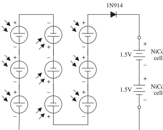
The circuit here shows how nine solar cells placed in series can be used to recharge two 1.5-V NiCd cells. (Each cell provides 0.5 V, so the total voltage is 4.5 V minus a 0.6-V drop due to the diode.) The diode is added to the circuit to prevent the NiCd cells from discharging through the solar cell during times of darkness. It is important not to exceed the safe charging rate of NiCd cells. To slow the charge rate, a resistor placed in series with the batteries can be added.
