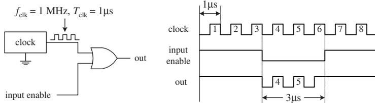
Below, an OR gate is used as the enable gate. The output is held high when the input enable lead is high, even as the clock signal is varying. However, when the enable input is low, the clock pulses are passed to the output.
