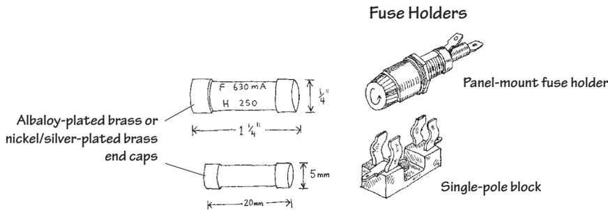
These are made by encapsulating a current-sensitive wire or ceramic element within a glass cylinder. Each end of the cylinder contains a metal cap that acts as a contact lead. Fuses may be fast-acting or time-lagging. They are used in instruments, electric circuits, and small appliances. Typical cylinders come in  $\frac{1}{4} \times 1\frac{1}{4}$  in or  $5 \times 20$  mm sizes. Current ratings range from around  $\frac{1}{4}$  to 20 A, with voltage ratings of 32, 125, and 250 V.
