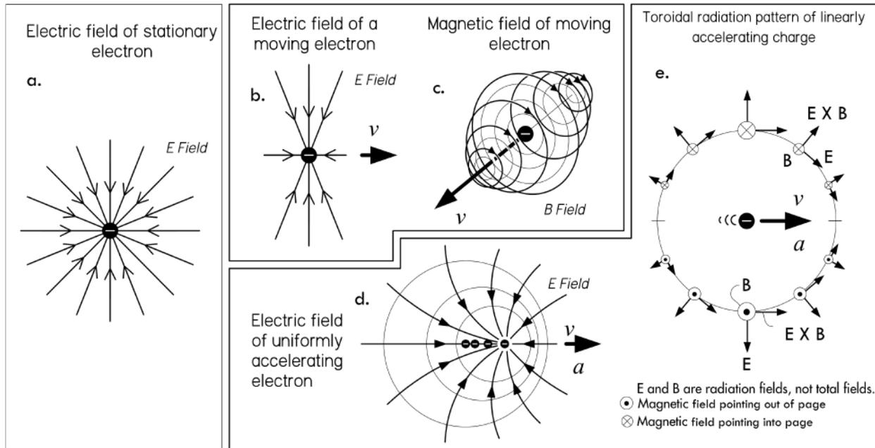
**FIGURE 2.110** The electric and magnetic fields are part of the same phenomenon called electromagnetism. Magnetic fields appear whenever a charge is in motion. Interestingly, if you move along with a moving charge, the observable magnetic field would disappear—thanks to Einstein’s relativity.
