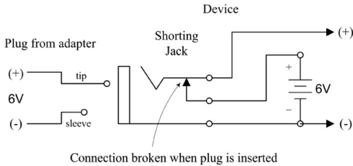
This figure shows a simple way to add an external dc power supply input to a battery-powered device. With no external power (external dc adapter plug not connected), the shunting jack acts to switch power to the battery. However, when external dc power is applied via a dc adapter plug, the shunting jack switches power from the battery to the dc adapter connects.
