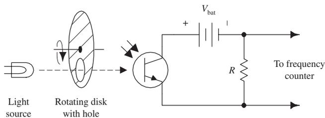
Here is a simple example of how a phototransistor can be used as a simple input stage for a frequency counter, or tachometer. A rotating disk with a hole (connected to a rotating shaft) will pass light through its hole once every revolution. The light that passes will then trigger the phototransistor into conduction. A frequency counter is used to count the number of electrical pulses generated.
