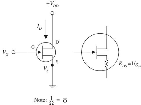
If  $V_{GS, \text{off}} = -4 \text{ V}$  and  $I_{DSS} = 12 \text{ mA}$ , find the values of  $I_D$  and  $g_m$  and  $R_{DS}$  when  $V_{GS} = -2 \text{ V}$  and when  $V_{GS} = +1 \text{ V}$ . Assume that the JFET is in the active region.
