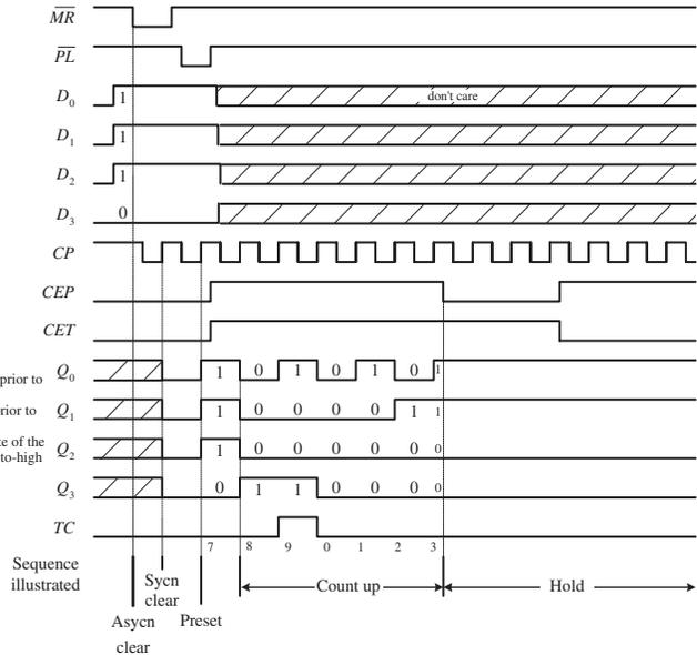
Synchronous multistage counter using the 74163
