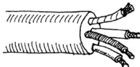
This type of cable consists of a number of individually wrapped, color-coded wires. It is used when a number of signals must be sent through one cable.
