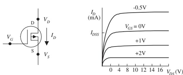
**CUTOFF VOLTAGE ( $V_{GS,OFF}$ )** Often referred to as the *pinch-off voltage* ( $V_p$ ). Represents the particular gate-source voltage that causes the MOSFET to block almost all drain-source current flow.
