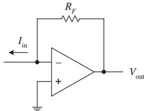
The circuit shown here transforms a current into a voltage. The feedback resistor  $R_F$  helps establish a voltage at the inverting input and controls the swing of the output. The output voltage for this circuit is given by
