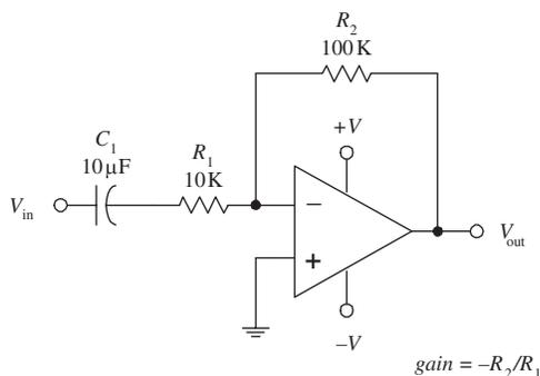
In both amplifier circuits,  $C_1$  acts as an ac coupling capacitor—it acts to pass ac signals while preventing unwanted dc signals from passing from the previous stage. Without  $C_1$ , dc levels would be present at the op amp's output, which in turn could lead to amplifier saturation and distortion as the ac portion of the input signal is amplified.  $C_1$  also helps prevent low-frequency noise from reaching the amplifier's input.
