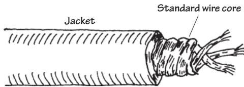
The main conductor is comprised of a number of individual strands of copper. Stranded wire tends to be a better conductor than solid-core wire because the individual wires together comprise a greater surface area. Stranded wire will not break easily when flexed.
