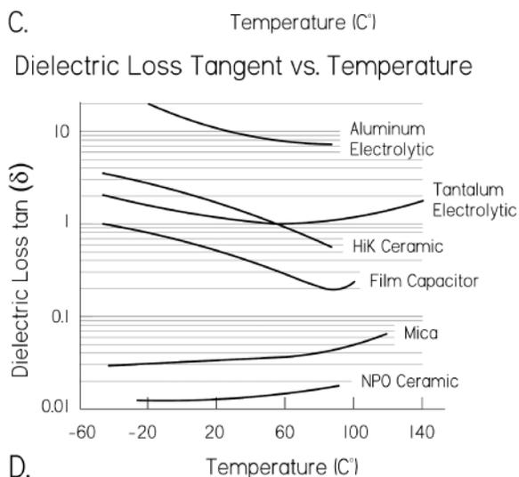
Graph D: Shows the dielectric loss tangent as a function of temperature for various capacitors.
