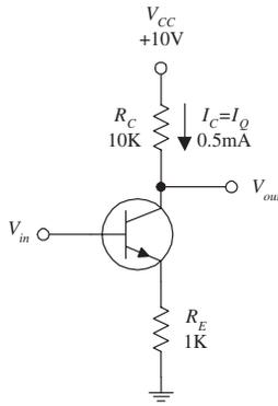
For example, if  $V_{CC}$  is 10 V and  $I_Q$  is 0.5 mA,  $R_C$  is then 10 k. The gain of this circuit is found by realizing that  $\Delta V_E = \Delta V_B$  (where  $\Delta$  represents a small fluctuation). The emitter current is found using Ohm's law:
