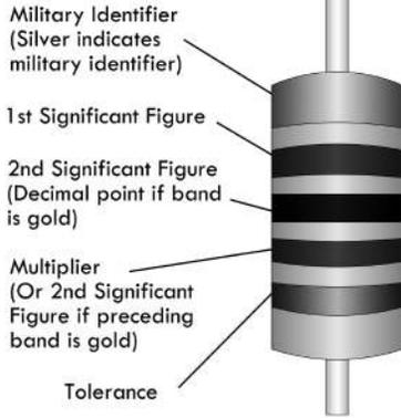
Axial-leaded inductors are typically color banded. The military color code consists of 5 bands. A silver band that is double the width of the other four bands is located near one end. When present, the band identifies military radio frequency coils. The next three bands indicate the inductance value in microhenries, while the fourth band indicates tolerance.
