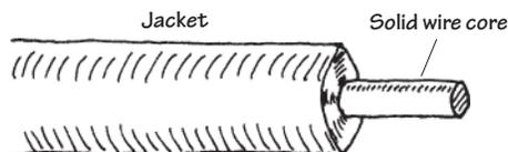
This wire is useful for wiring breadboards; the solid-core ends slip easily into breadboard sockets and will not fray in the process. These wires have the tendency to snap after a number of flexes.
