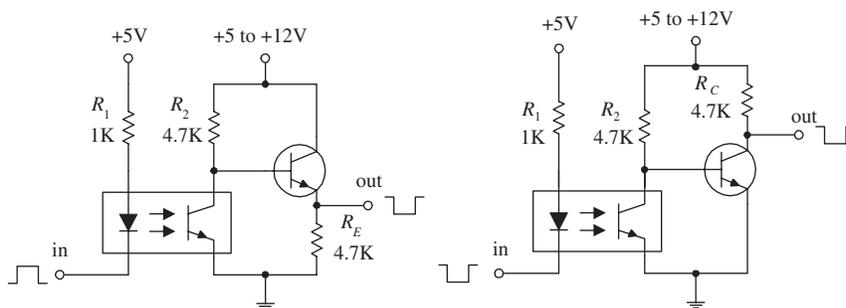
In optoelectronic applications, the phototransistor section of an optoisolator may not be able to provide enough power-handling capacity to switch large currents. The circuits to the right incorporate a power-switching transistor to solve this problem.
