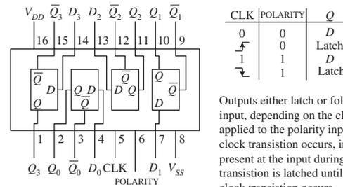
Outputs either latch or follow the data input, depending on the clock level applied to the polarity input. When clock transition occurs, information present at the input during the clock transition is latched until an opposite clock transition occurs.
