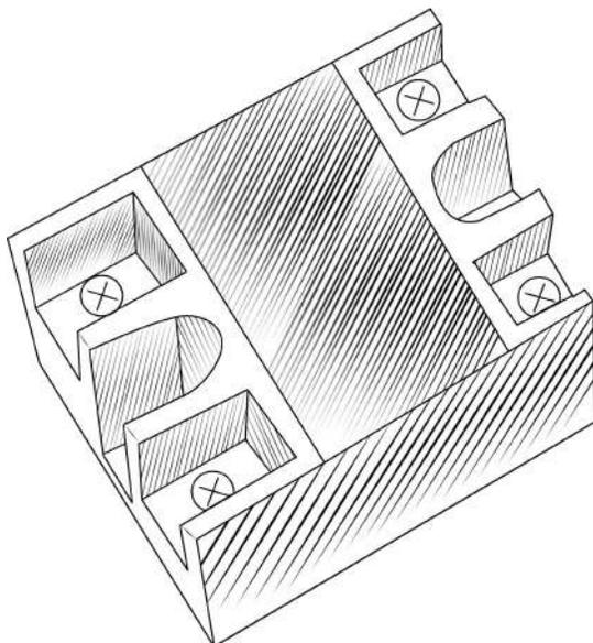
Solid-State Relays or SSRs are sealed modules designed to be used in the same way as electromechanical relays, but switching using opto-isolators and power transistors or Triacs. As such they are not really basic components, but modules.
