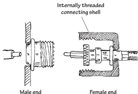
F-type connectors are used with a variety of unbalanced coaxial cables. They are commonly used to interconnect video components. F-type connectors are either threaded or friction-fit together.
