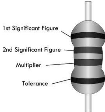
The 4-band color code does not contain a military band. The first and second bands represent first and second significant figures. The third band represents the multiplier, where silver = x 0.01, and gold = x 0.1. The fourth band indicates the tolerance, where black is ±20%, silver is ±10%, and gold is ±5%. All values are given in microhenries.
