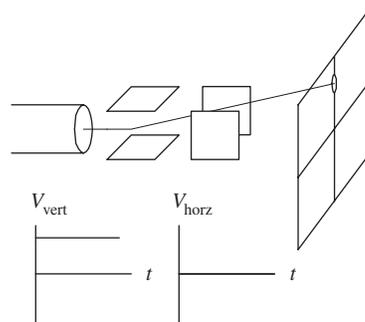
When a dc voltage is applied to the vertical plates, while no voltage is applied to the horizontal plates, the electron beam shifts up or down depending on the sign of the applied voltage.
