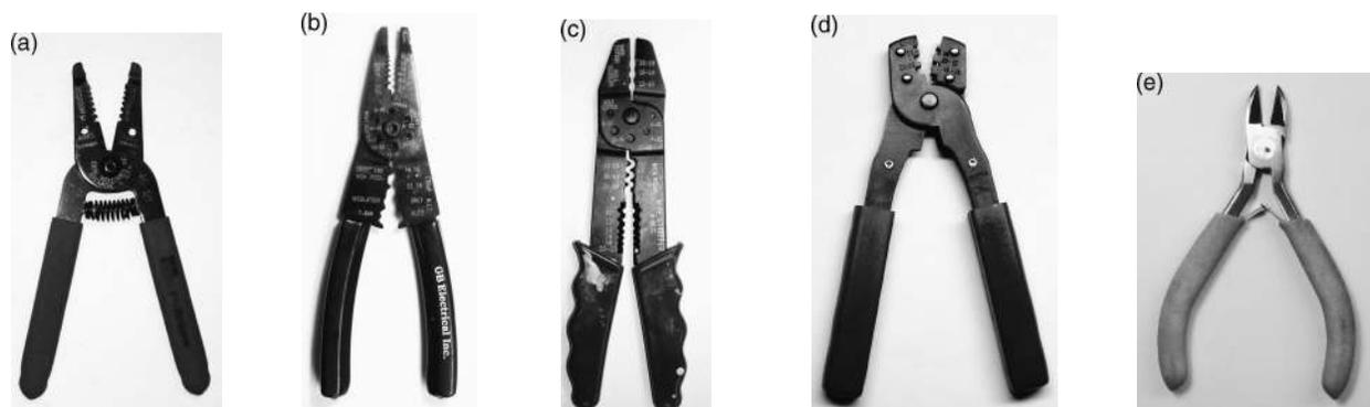
FIGURE 7.73 (a) Stripper (16–26 AWG). (b and c) Solderless crimping tools with additional features. (d) D-Sub crimping tool. (e) Diagonal cutter.
