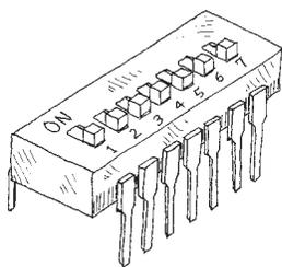
DIP stands for “dual-inline package.” The geometry of this switch’s pin-outs allows the switch to be placed in IC sockets that can be wired directly into a circuit board.
