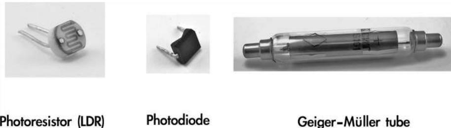
FIGURE 6.26 Light, radiation, and magnetic sensors.
