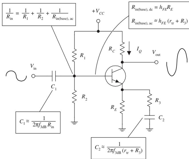
The circuit shown here is known as a *common-emitter amplifier*. Unlike the common-collector amplifier, the common-emitter amplifier provides voltage gain. This amplifier makes use of the common-emitter arrangement and is modified to allow for ac coupling. To understand how the amplifier works, let's go through the following example.
