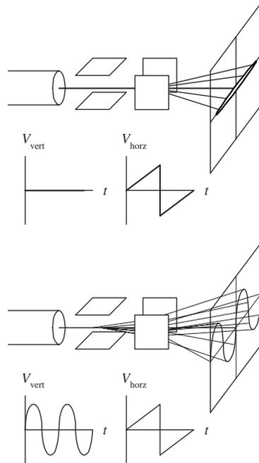
When a dc voltage is applied to the vertical plates, while a sawtooth voltage is applied to the horizontal plates, a horizontal line is created that is shifted up or down depending on the sign of the dc vertical plate voltage (+ or -).
