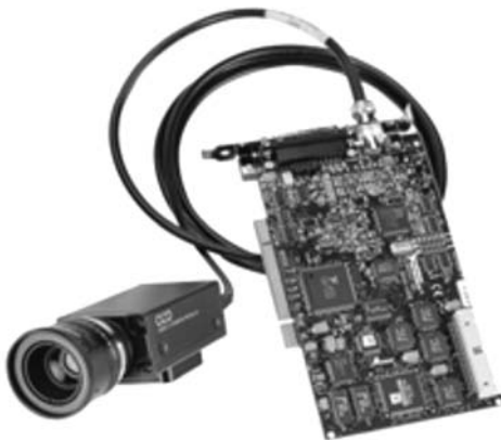
Figure 1.8 Analog camera connected to an analog frame grabber card with a BNC cable. Video standards for color and monochrome analog camera are summarized in Table 1.4.
