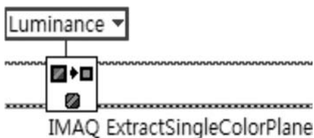
Figure 3.25 Extracting the luminance plane of a color image for conversion to a grayscale image.
