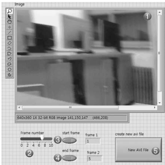
Figure 16.12 Front panel of VI to create a new AVI file from the existing AVI file.
