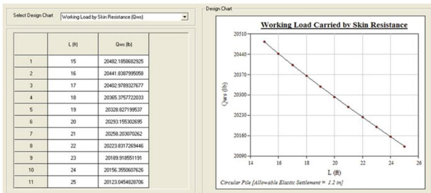
Fig. 2.28 Skin friction resistance results based on settlement analyses
