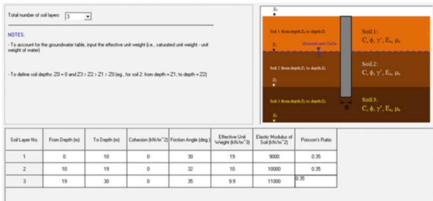
**Fig. 2.29** Thicknesses and physical properties of soil layers
