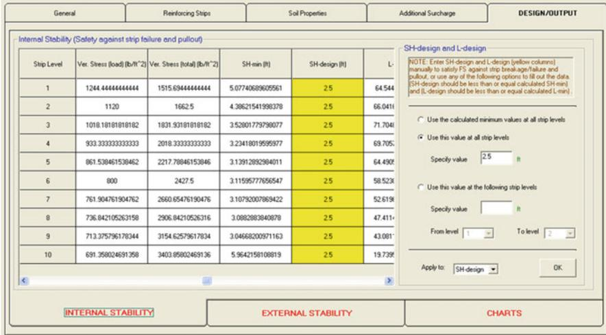
Fig. 4.32 DESIGN/OUTPUT section (design of horizontal spacing—internal stability)
