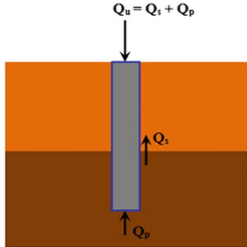
**Calculation of Pile Tip Resistance - End Bearing ( $Q_p$ )**
