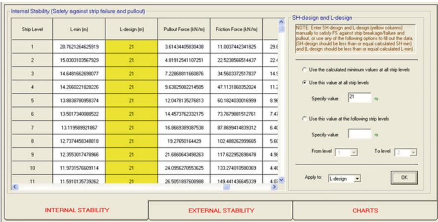
Fig. 4.11 DESIGN/OUTPUT section (design of strip length—internal stability)
