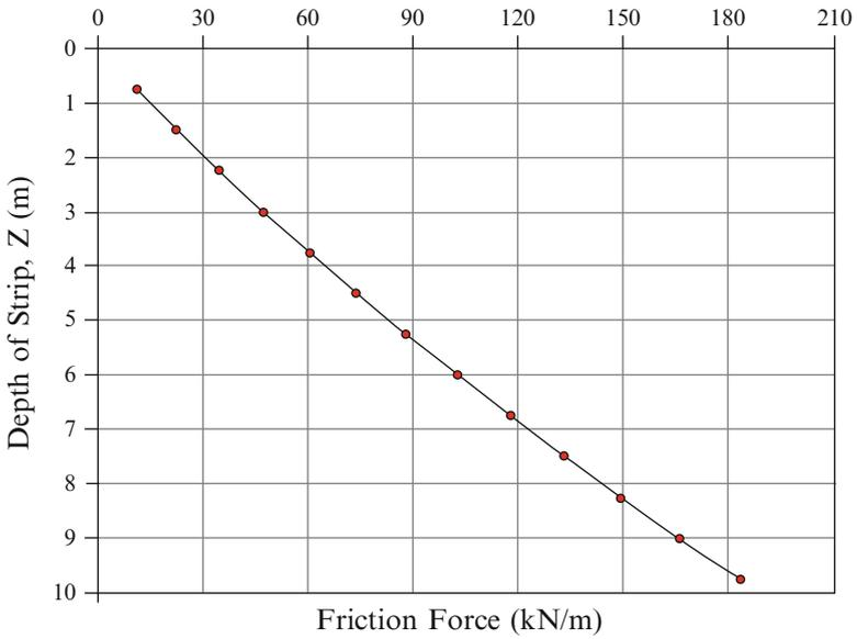
Fig. 4.16 Distribution of the maximum pullout/friction forces
