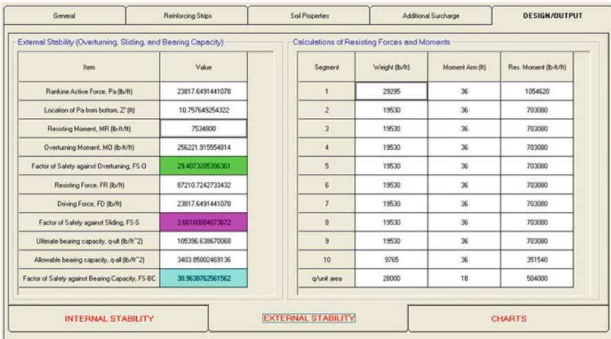
Fig. 4.34 DESIGN/OUTPUT section (external stability)
