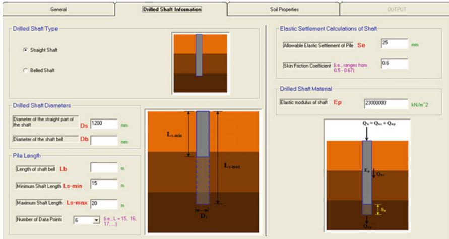
Fig. 3.6 The Drilled Shaft Information section for Shaft-1 application
