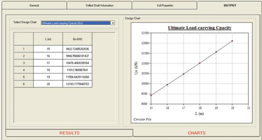
Fig. 3.9 Ultimate axial capacity design chart—OUTPUT section (Chart format)
