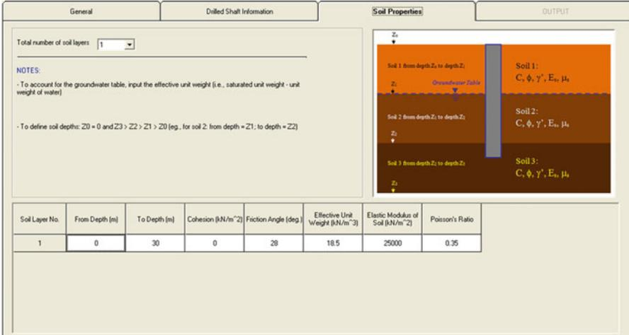
Fig. 3.7 Soil Properties section for Shaft-1 application
