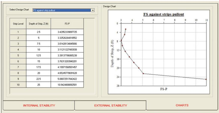
Fig. 4.36 Distribution of safety factor against pullout for the selected design parameters
