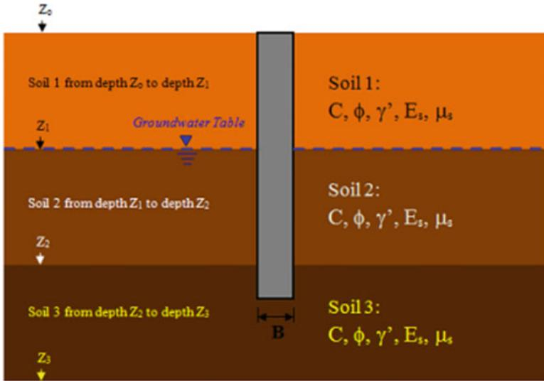
Fig. 2.1 Single pile embedded in multiple soil layers
