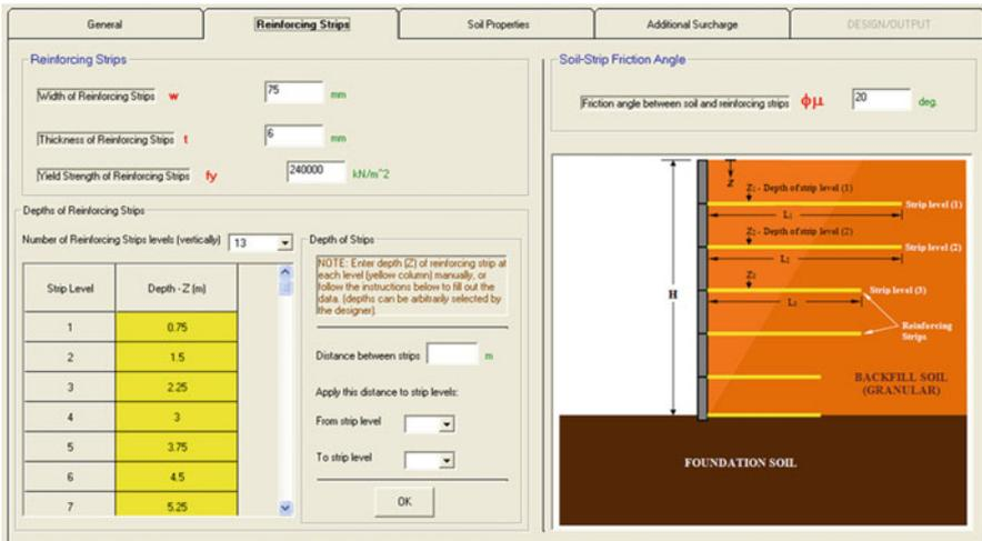
Fig. 4.7 Reinforcing Strips section
