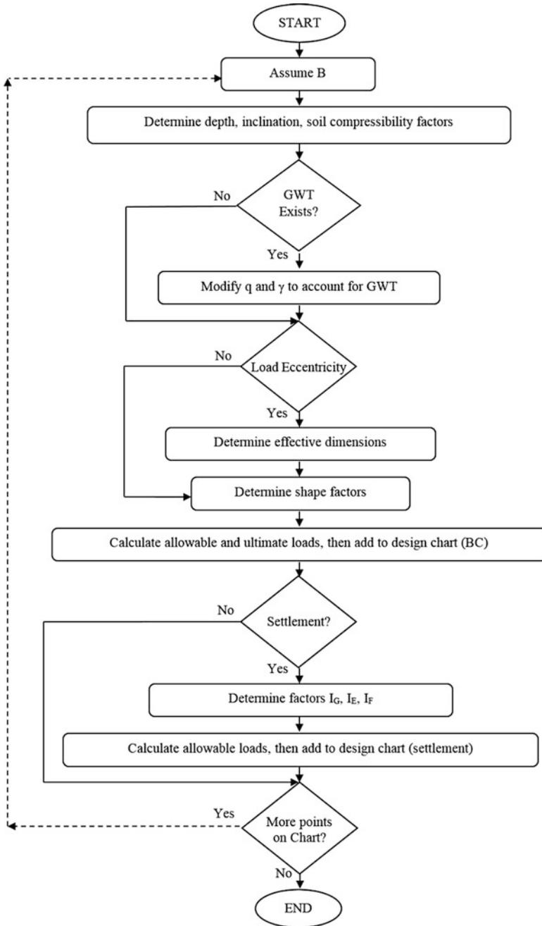
Fig. 1.7 Flowchart for development of design capacity charts
