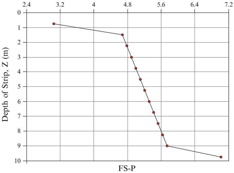
Fig. 4.18 Distribution of safety factor against pullout for the selected design parameters
