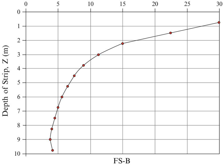
Fig. 4.17 Distribution of safety factor against breakage for the selected design parameters
