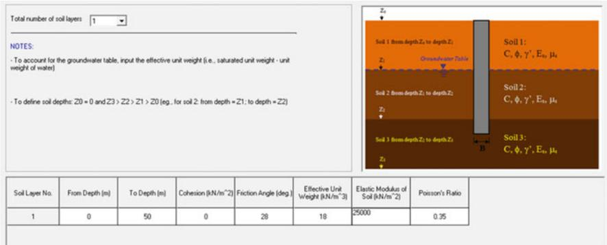
Fig. 2.9 Properties and thicknesses of soil layers
