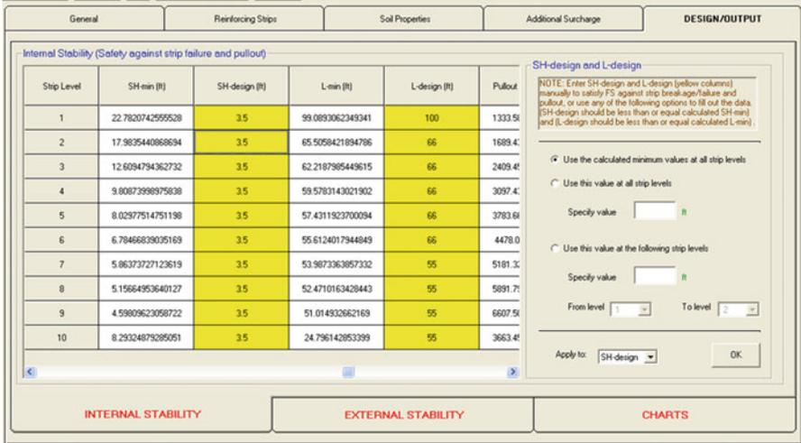
Fig. 4.38 Design of horizontal spacing and strip length—internal stability
