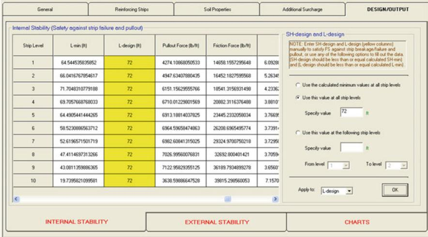
Fig. 4.33 DESIGN/OUTPUT section (design of strip length—internal stability)
