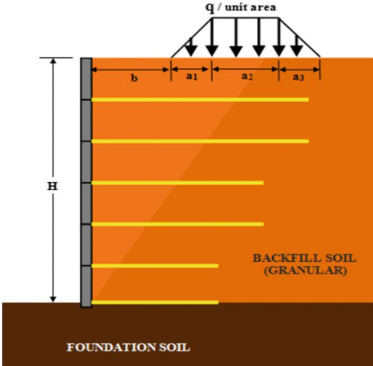
Fig. 4.4 Analysis of MSE wall with an embankment load
