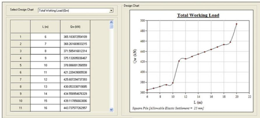
Fig. 3.25 A snapshot from the OUTPUT section of the Shaft-1 application
