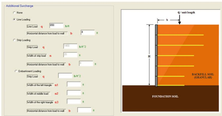
Fig. 4.37 Additional Surcharge Loading section
