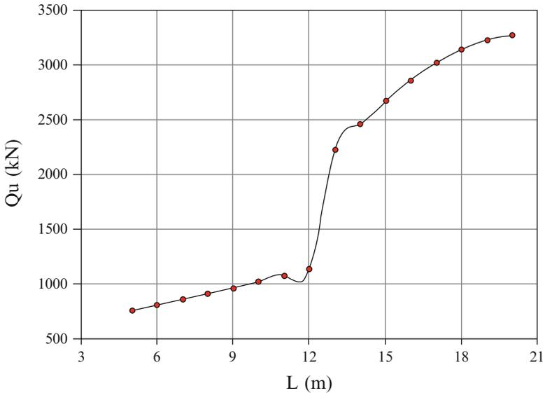
**Fig. 2.32** Ultimate load carrying capacity design chart (bearing capacity analysis)
