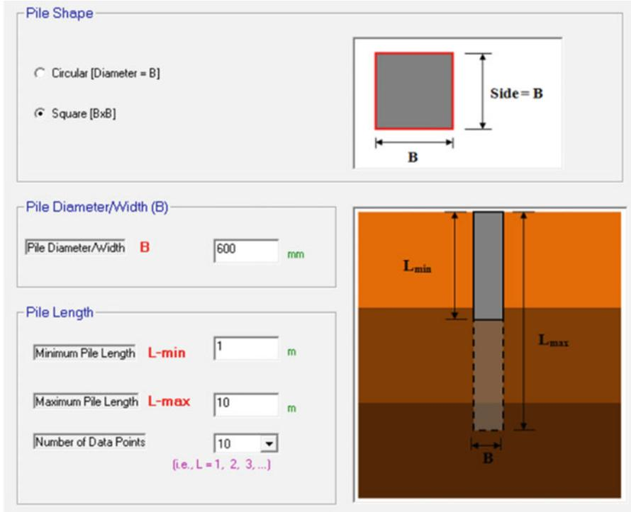
Fig. 2.20 Pile Information section
