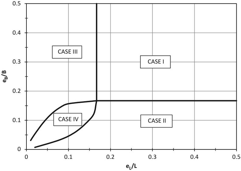
**Fig. 1.5** Two-way load eccentricity cases
