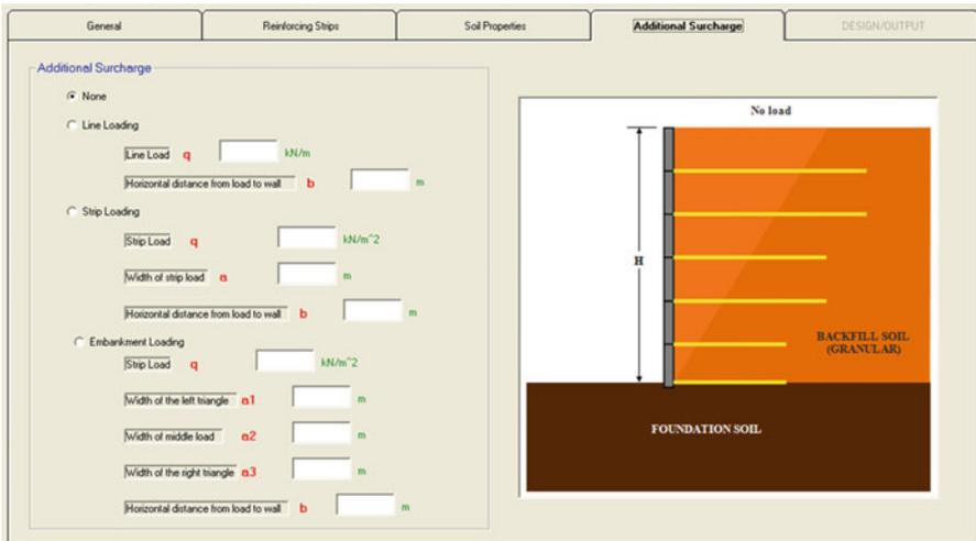
Fig. 4.22 Additional Surcharge Loading section
