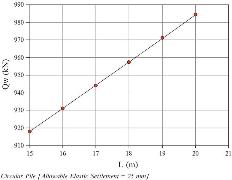
Fig. 3.10 Total working load design chart
