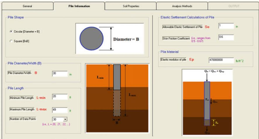
Fig. 2.34 Pile Information section
