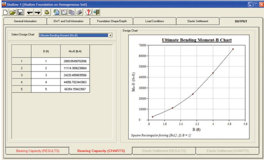
Fig. 1.34 Ultimate bending moment in the  $B$ -direction
