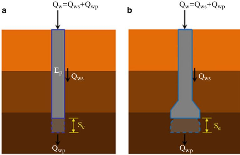
**Fig. 3.3** Definition of working loads due to total settlement for (a) straight shaft and (b) belled shaft
