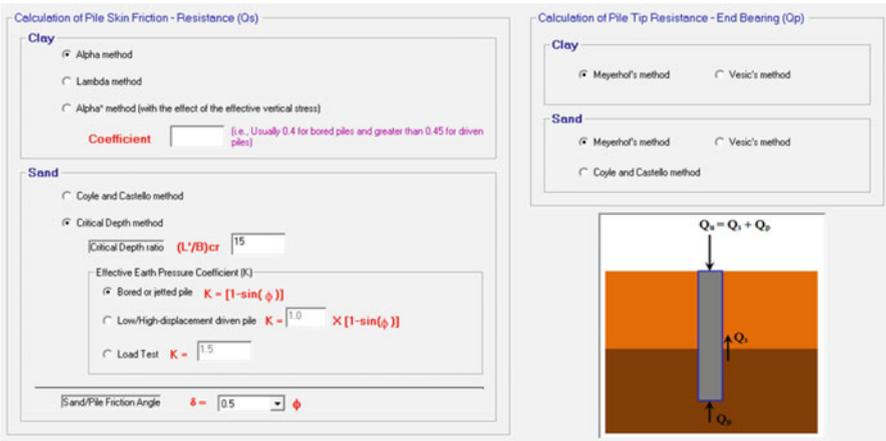
Fig. 2.10 Analysis Methods section for Pile-1 application
