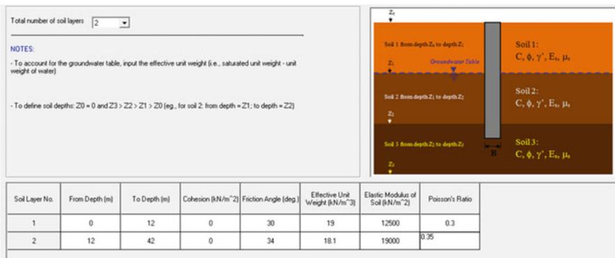
Fig. 2.31 Properties of sand layers
