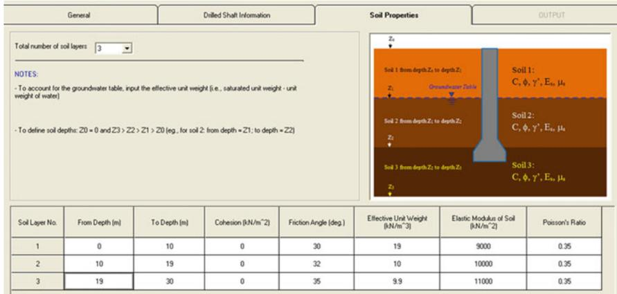
Fig. 3.23 Physical properties and thicknesses of sand layers
