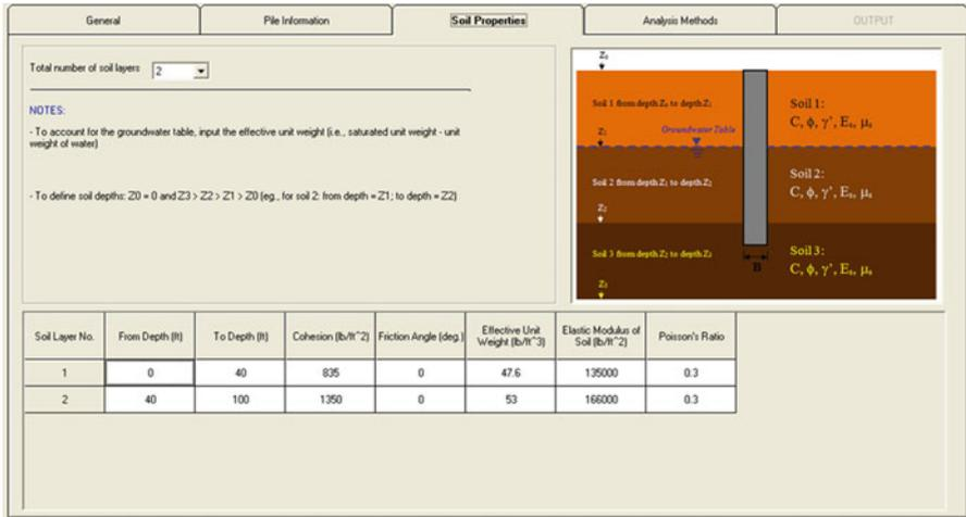
Fig. 2.35 Soil properties used for this design problem
