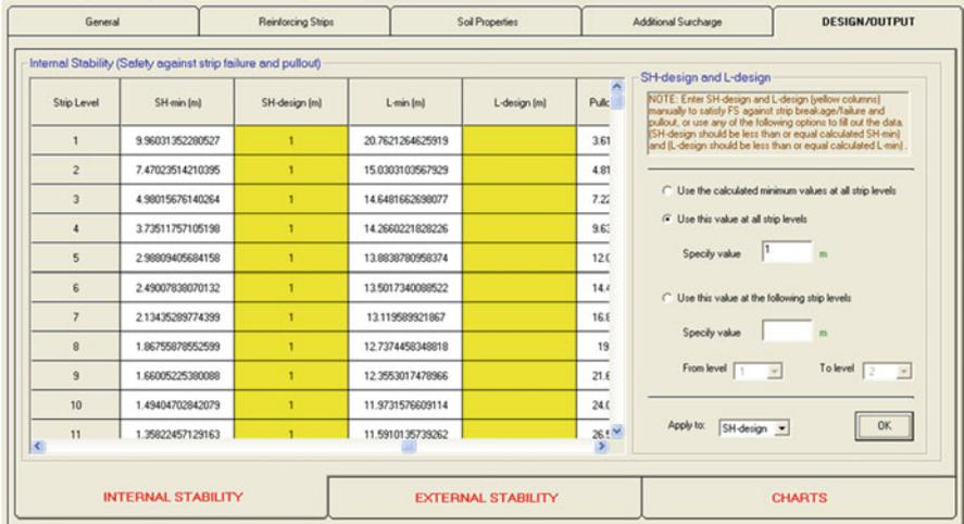
Fig. 4.10 DESIGN/OUTPUT section (design horizontal spacing—internal stability)
