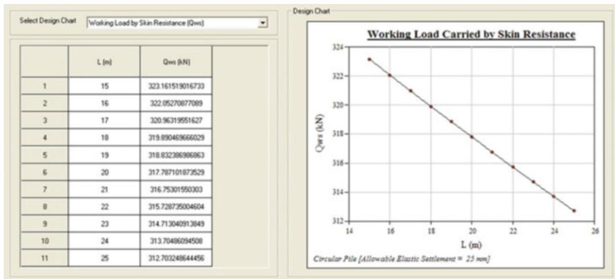
Fig. 3.15 Results of working load carried by skin friction component
