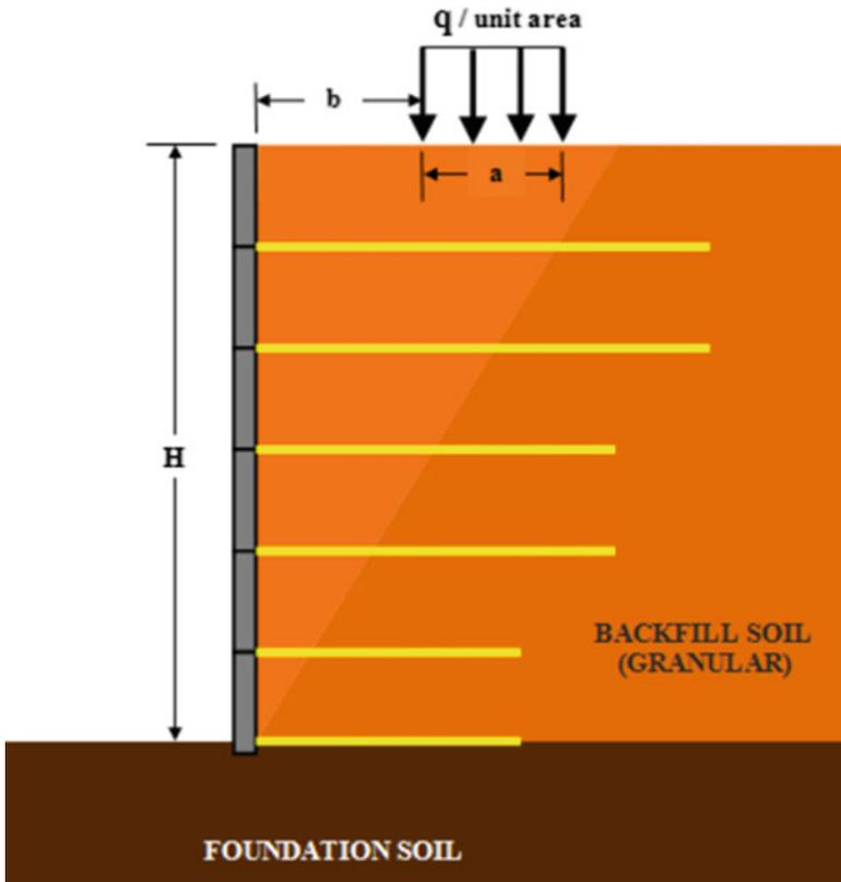
Fig. 4.3 Analysis of MSE wall with a strip load
