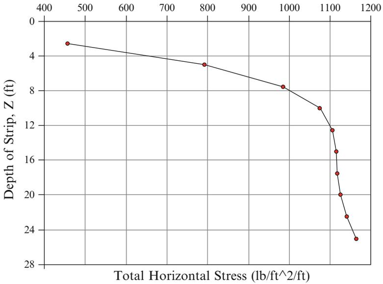
Fig. 4.35 Distribution of total horizontal stresses due to soil and strip loading
