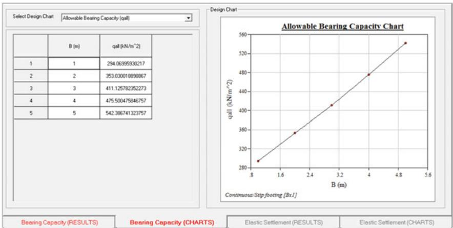
Fig. 1.13 Bearing capacity results (chart format)
