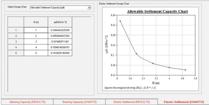
Fig. 1.38 Allowable settlement capacity results
