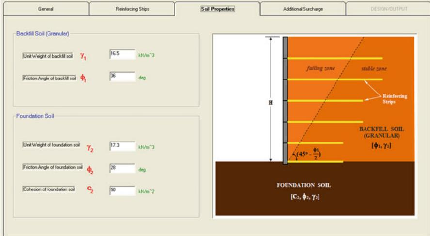
Fig. 4.8 Soil Properties section
