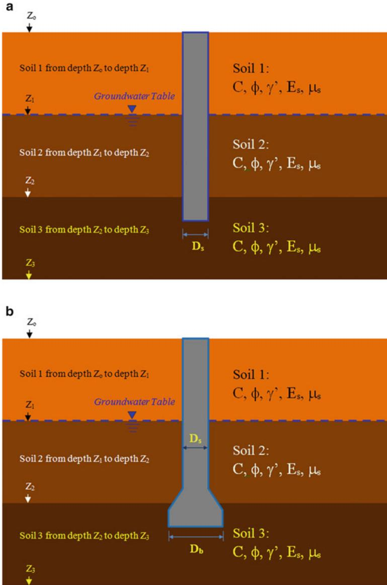
**Fig. 3.1** Single drilled shaft embedded in multiple soil layers: (a) straight shaft and (b) belled shaft
