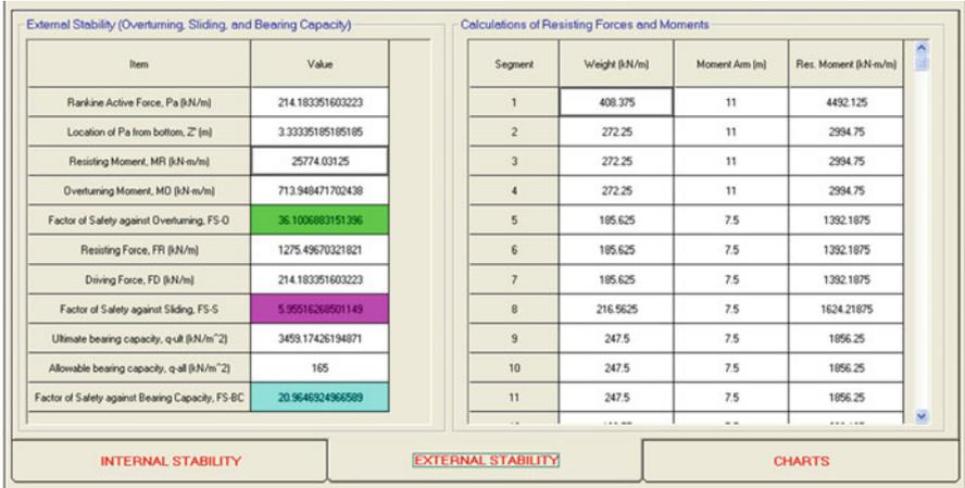
Fig. 4.25 DESIGN/OUTPUT section (external stability)
