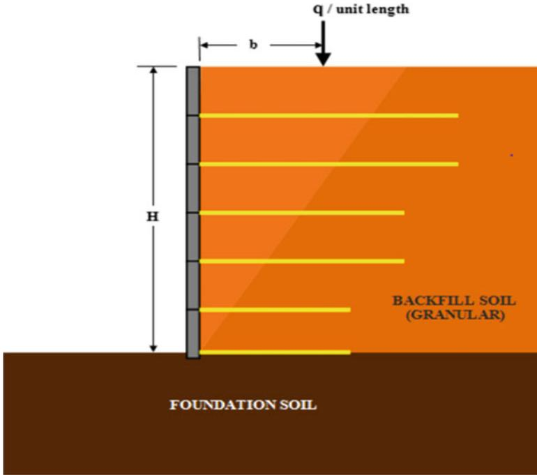
Fig. 4.2 Analysis of MSE wall with a line load
