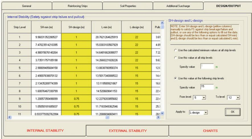
Fig. 4.24 DESIGN/OUTPUT section (design of strip length—internal stability)
