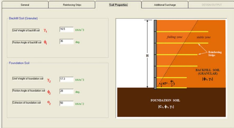
Fig. 4.21 Soil Properties section
