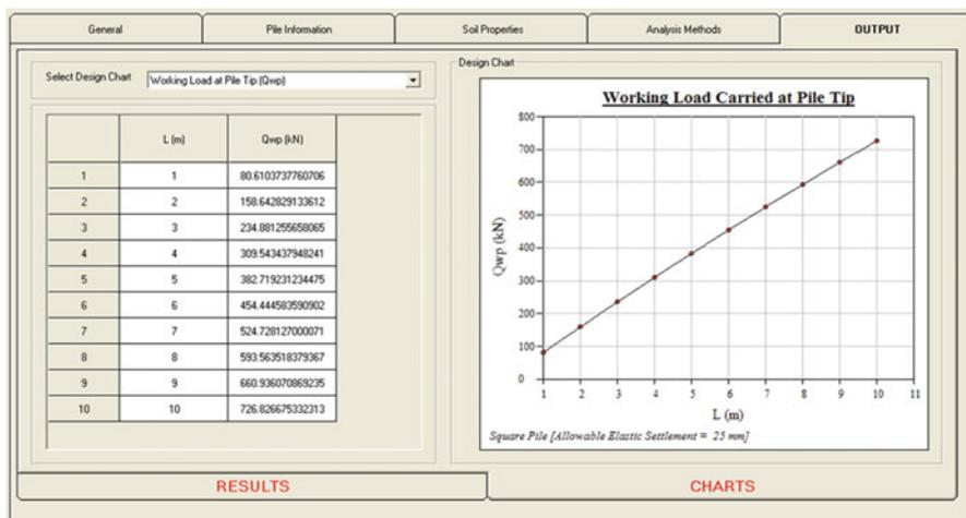
**Fig. 2.21** A snapshot of one of the design charts from Pile-1 application
