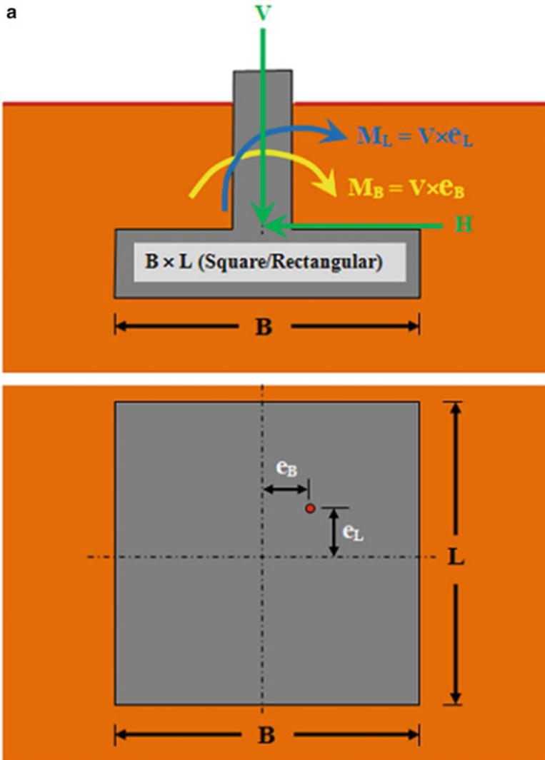
**Fig. 1.4** Load eccentricity cases and application of bending moment: (a) Application of bending moments on square/rectangular foundation; (b) application of bending moments on circular foundation; (c) application of bending moments on strip/continuous foundation
