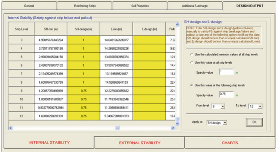
Fig. 4.23 DESIGN/OUTPUT section (design of horizontal spacing—internal stability)
