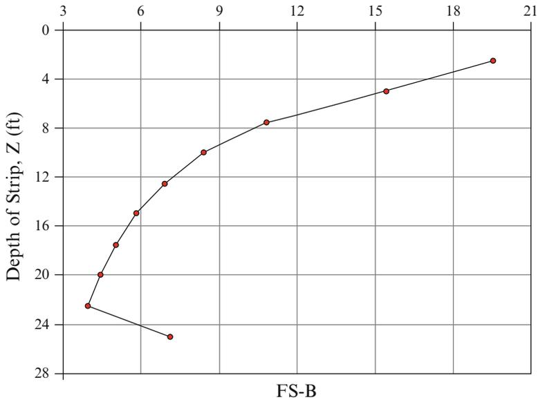
**Fig. 4.40** Distribution of safety factors against strip breakage
