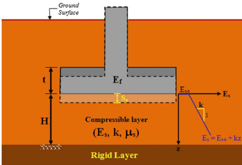
Fig. 1.6 Elastic settlement of shallow foundation
