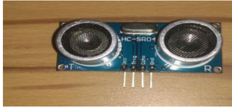
Figure 18.1 Ultrasonic Sensor Working
