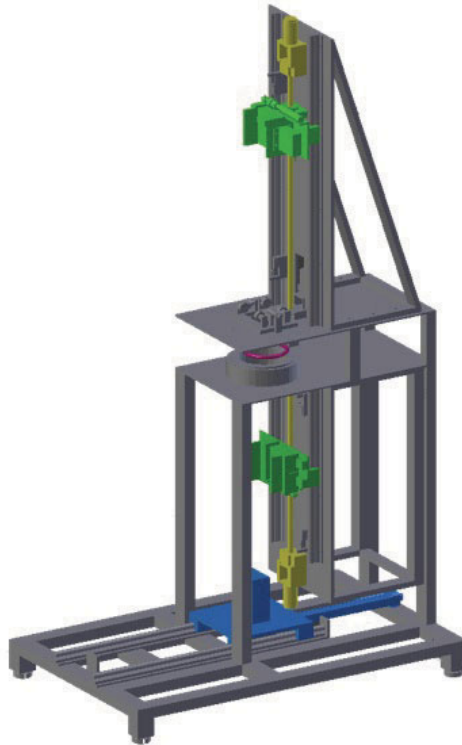
Figure 11.1 Proposed mechanical structure of Ro CIF VIP with 5 DOF
