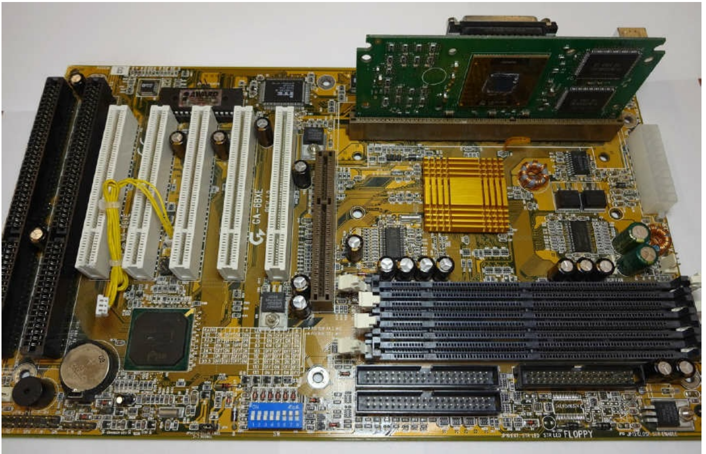
Figure 1.4: PC circuit board, circa 1998; 12 \times 7.5 inches ( 30 \times 19 cm).
