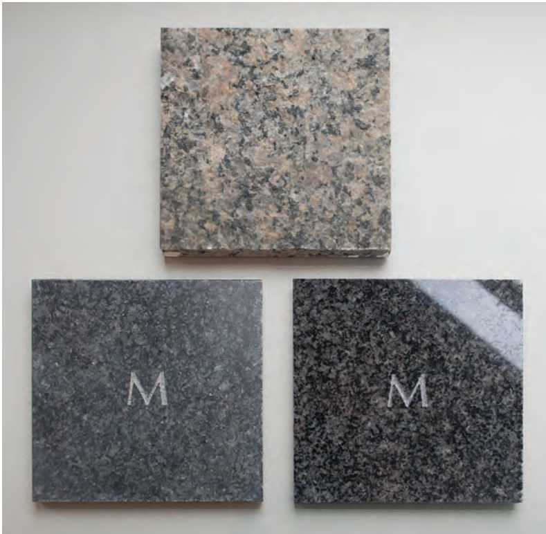
6.71 Stone finishes: Top, thermal finished granite has a rough surface texture; Bottom, color difference between honed and polished samples of the same granite.
