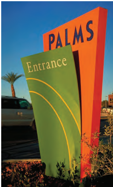
6.34 A metal panel is rolled into a simple, graceful curve on this sign for the Palms Casino in Las Vegas.
