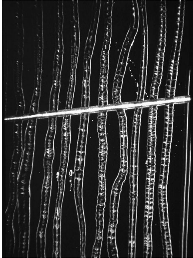
Figure 7.4 A human hair laid across the groove offers a point of reference for size.
