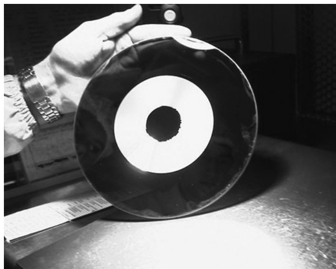
Figure 6.2 A glass master with a CD image in the center. (Image courtesy of DVDBits.com.)
