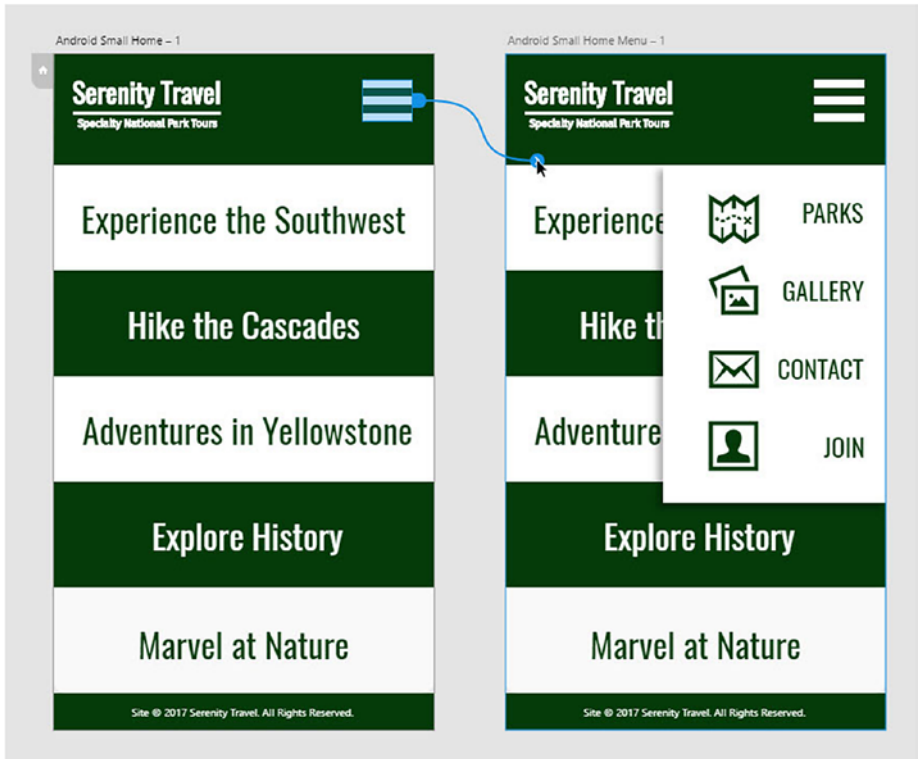
Figure 9-6. Simulating a drop-down menu by linking the hamburger icon to an artboard that shows the menu
